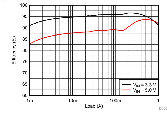
図 8. 2.5-V Output Efficiency
