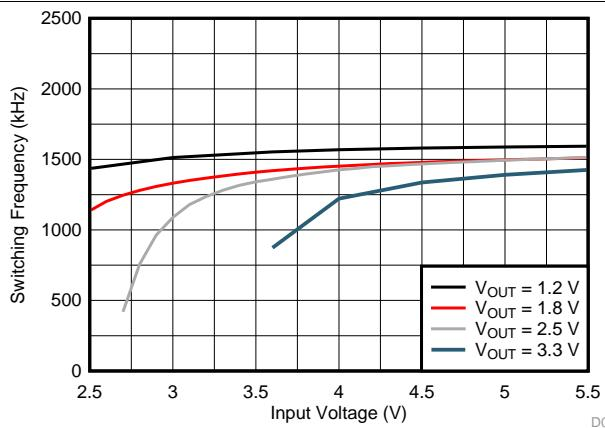
図 13. Switching Frequency vs Input Voltage
