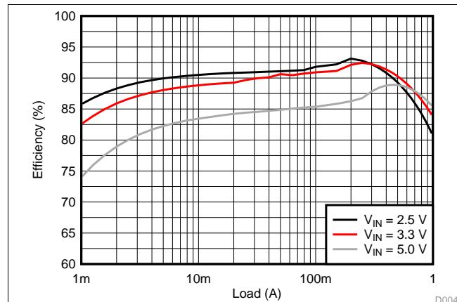
図 6. 1.2-V Output Efficiency
