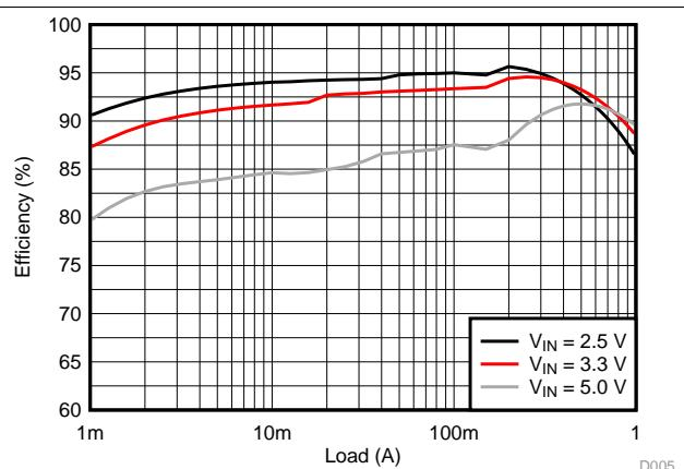
図 7. 1.8-V Output Efficiency
