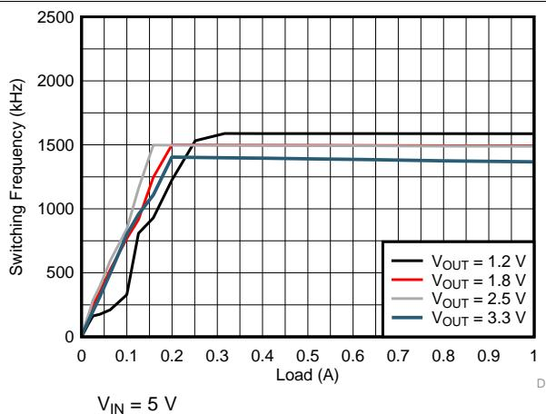
図 12. Switching Frequency vs Load
