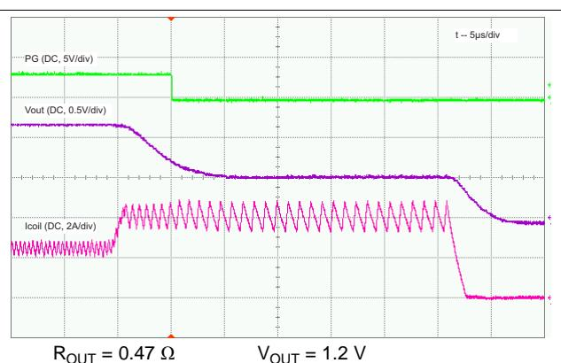
**図 22. Output Short-Circuit Protection, HICCUP Zoom In**
