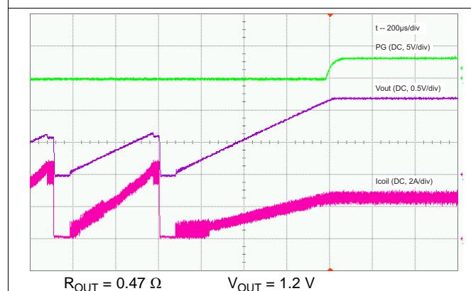
**図 21. Output Short-Circuit Protection, Recovery**
