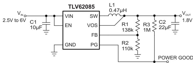
図 4. 1.8-V Output Voltage Application
