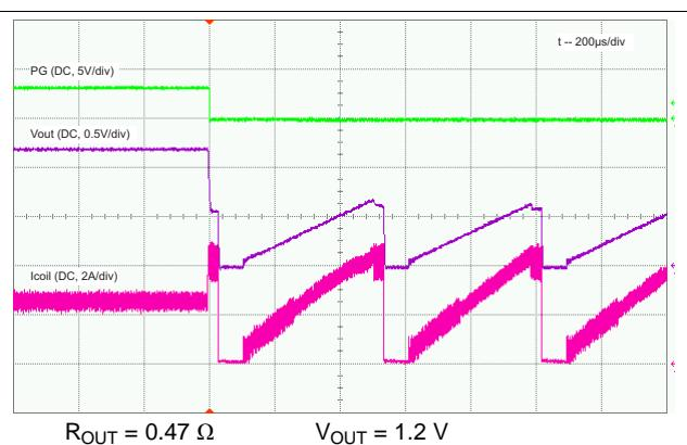
**図 20. Output Short-Circuit Protection, Entry**
