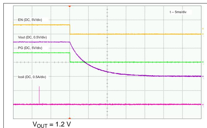
**図 17. Shutdown without Load**
