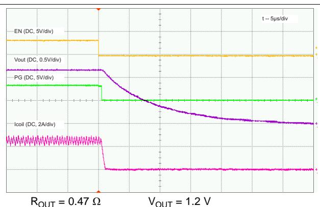
**図 16. Shutdown with Load**
