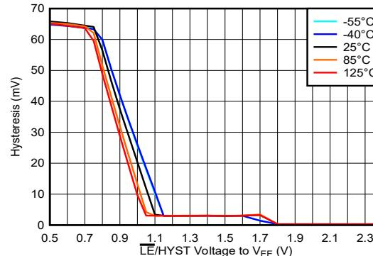
図 7-4. Hysteresis vs.  $V_{HYS}$  at  $V_{CC} = 5V$
