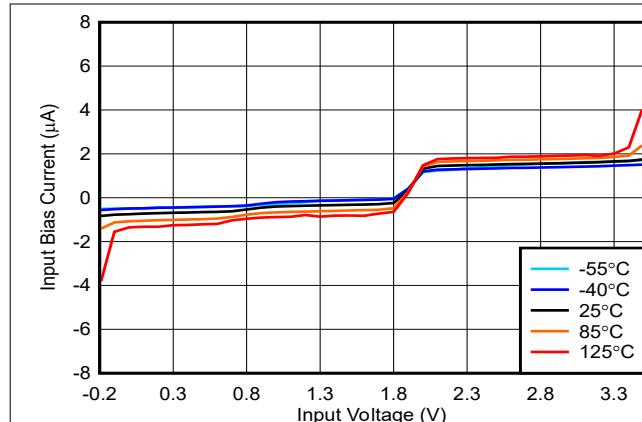
图 5-15. Bias Current vs. Input Voltage, 3.3V
