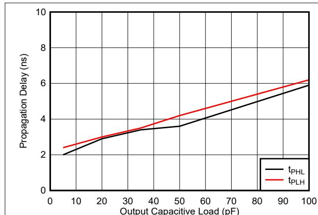
图 5-33. Propagation Delay vs. Load Capacitance, 3.3V
