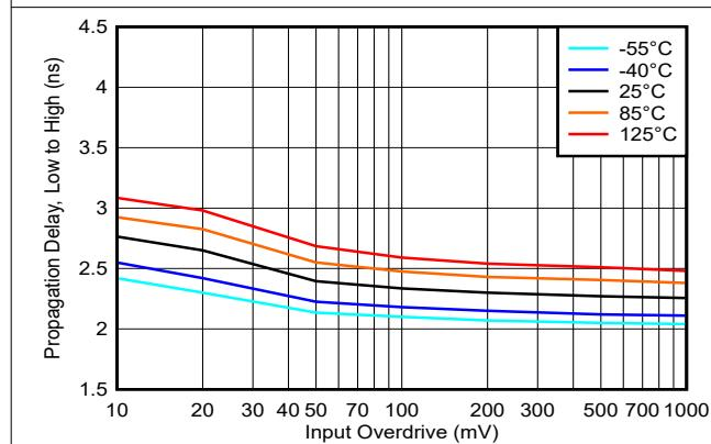
图 5-29. Propagation Delay, Low to High, 3.3V
