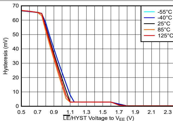
图 5-36. Hysteresis Voltage vs. LE/HYST Voltage, 2.5V
