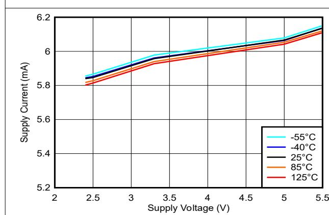
图 5-23. Supply Current vs. Voltage (Output Low)
