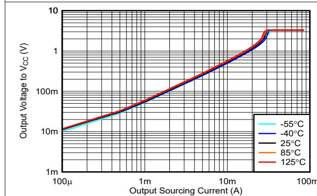
图 5-19. Output Voltage vs. Output Sourcing Current, 3.3V
