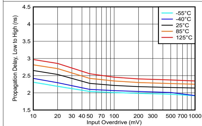
图 5-31. Propagation Delay, Low to High, 5V
