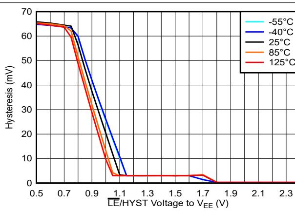
图 5-38. Hysteresis Voltage vs. LE/HYST Voltage, 5V
