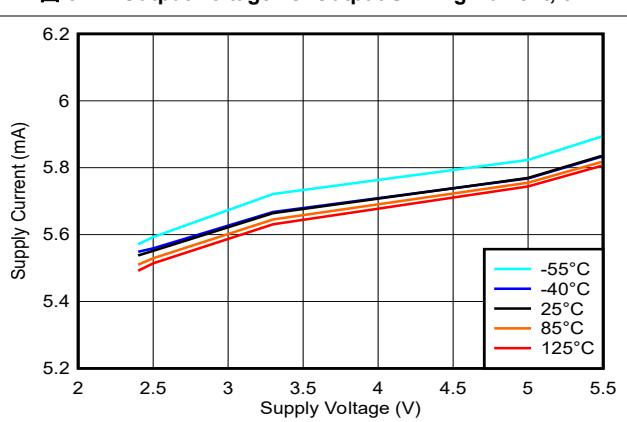
图 5-24. Supply Current vs. Voltage (Output High)
