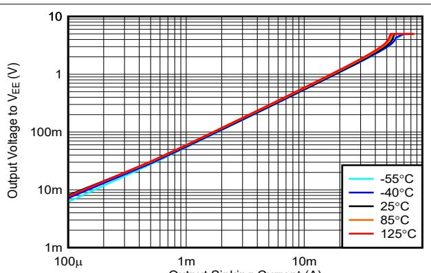
图 5-22. Output Voltage vs. Output Sinking Current, 5V
