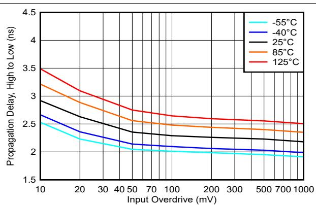
图 5-30. Propagation Delay, High to Low, 3.3V
