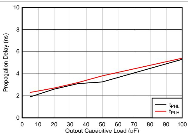
图 5-34. Propagation Delay vs. Load Capacitance, 5V
