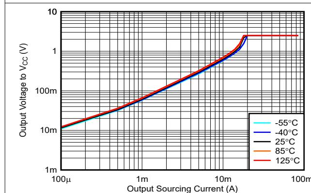
图 5-17. Output Voltage vs. Output Sourcing Current, 2.5V
