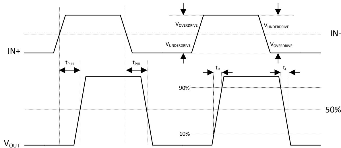
图 5-1. General Timing Diagram
