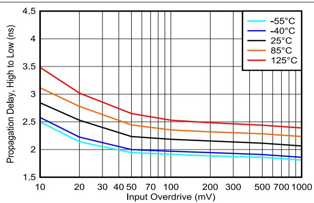
图 5-32. Propagation Delay, High to Low, 5V
