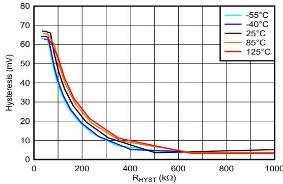
図 7-3. Hysteresis vs.  $R_{HYS}$  at  $V_{CC} = 5V$
