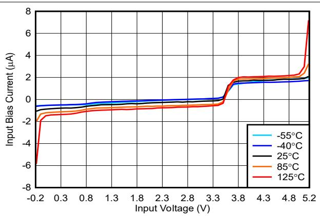
图 5-16. Bias Current vs. Input Voltage, 5V
