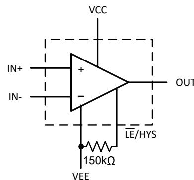
图 7-8. Setting the Hysteresis using a Resistor using the TLV3603-EP
