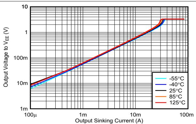
图 5-20. Output Voltage vs. Output Sinking Current, 3.3V
