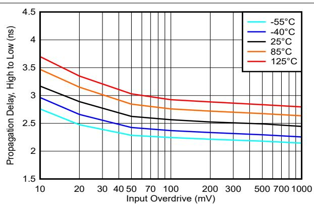
图 5-28. Propagation Delay, High to Low, 2.5V
