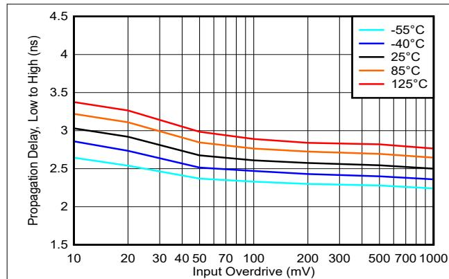
图 5-27. Propagation Delay, Low to High, 2.5V
