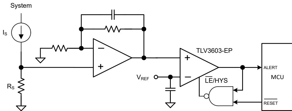
图 7-11. Over-Current Latched Output Circuit
