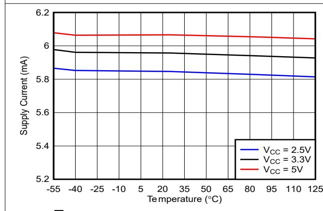
图 5-25. Supply Current vs. Temp (Output Low)
