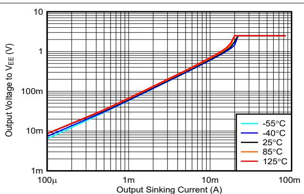
图 5-18. Output Voltage vs. Output Sinking Current, 2.5V
