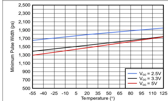
图 5-35. Minimum Pulse Width vs. Temperature
