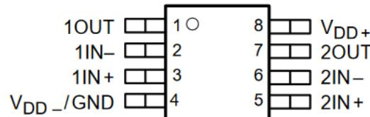
Figure 3-2. TLV2432x: PW Package, 8 Pin TSSOP
