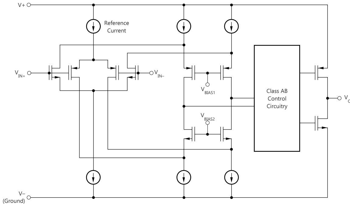
**Figure 5-1. Equivalent Schematic (Each Amplifier)**
