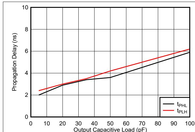
図 5-33. Propagation Delay vs. Load Capacitance, 3.3V
