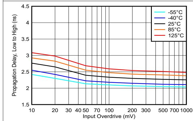
図 5-29. Propagation Delay, Low to High, 3.3V
