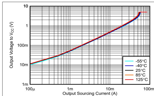
图 5-21. Output Voltage vs. Output Sourcing Current, 5V
