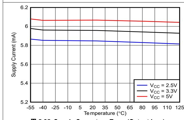
图 5-25. Supply Current vs. Temp (Output Low)
