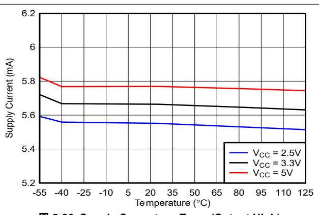
图 5-26. Supply Current vs. Temp (Output High)
