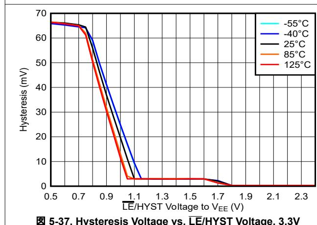
図 5-37. Hysteresis Voltage vs. LE/HYST Voltage, 3.3V
