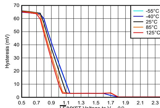
図 7-4. Hysteresis vs.  $V_{HYS}$  at  $V_{CC} = 5V$
