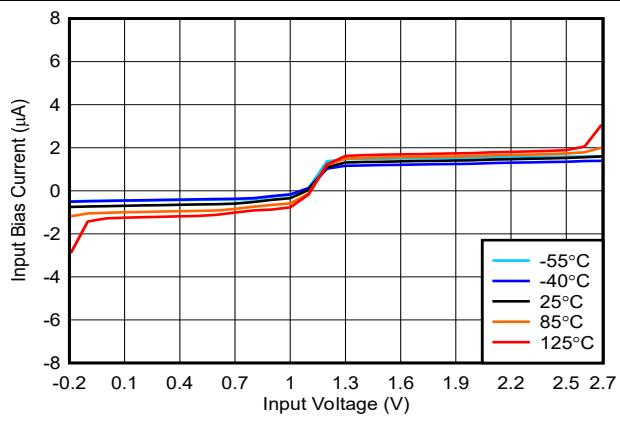
図 5-14. Bias Current vs. Input Voltage, 2.5V
