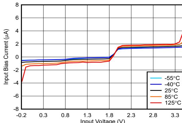
図 5-15. Bias Current vs. Input Voltage, 3.3V
