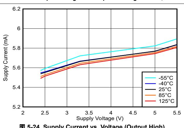
图 5-24. Supply Current vs. Voltage (Output High)
