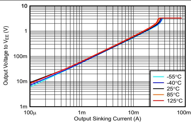
図 5-20. Output Voltage vs. Output Sinking Current, 3.3V
