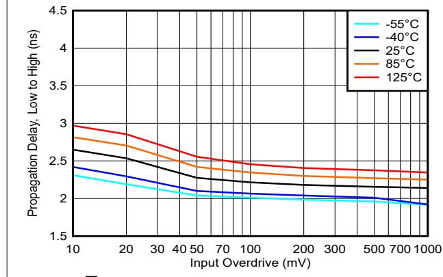
図 5-31. Propagation Delay, Low to High, 5V
