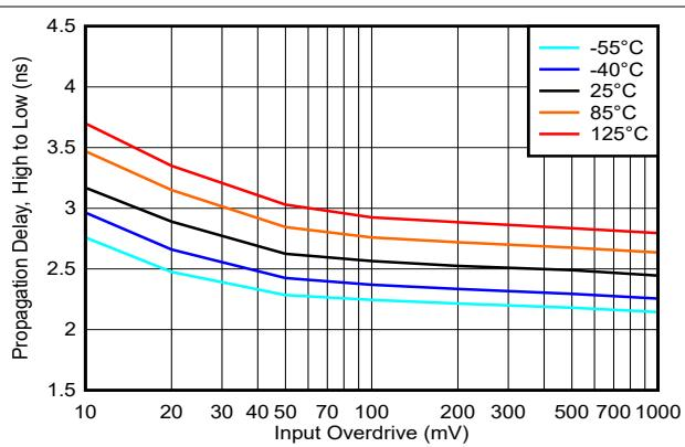
図 5-28. Propagation Delay, High to Low, 2.5V
