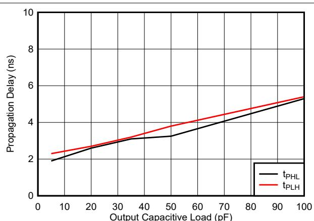
図 5-34. Propagation Delay vs. Load Capacitance, 5V
