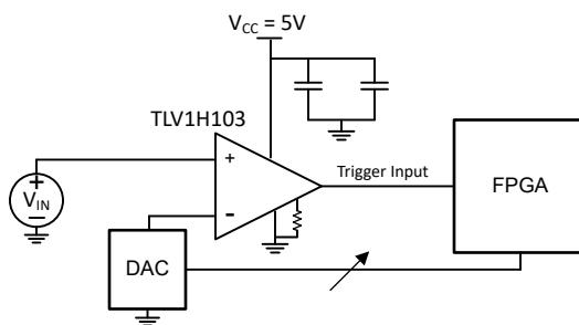
図 7-11. External Trigger Function
