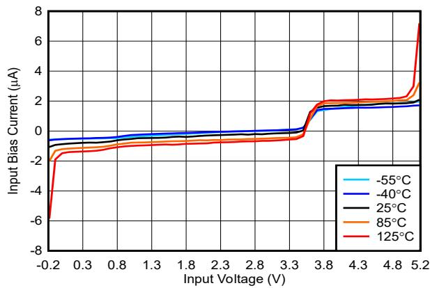
図 5-16. Bias Current vs. Input Voltage, 5V
