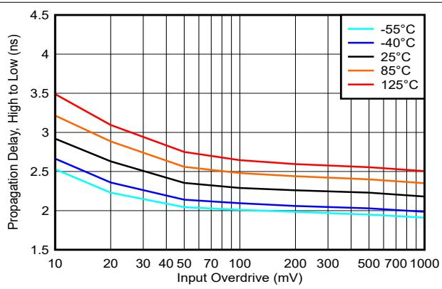
図 5-30. Propagation Delay, High to Low, 3.3V
