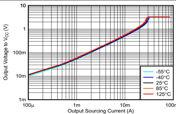
図 5-19. Output Voltage vs. Output Sourcing Current, 3.3V
