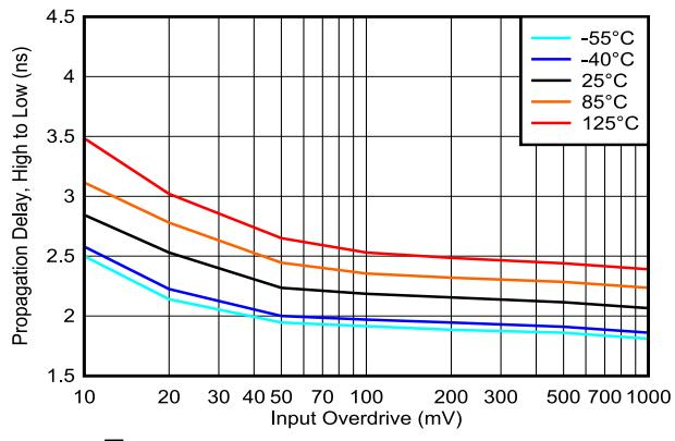
図 5-32. Propagation Delay, High to Low, 5V
