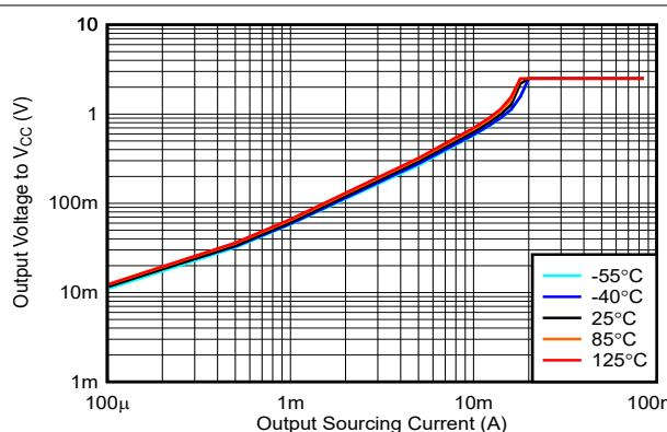
図 5-17. Output Voltage vs. Output Sourcing Current, 2.5V
