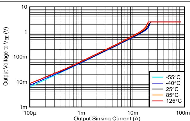
図 5-18. Output Voltage vs. Output Sinking Current, 2.5V
