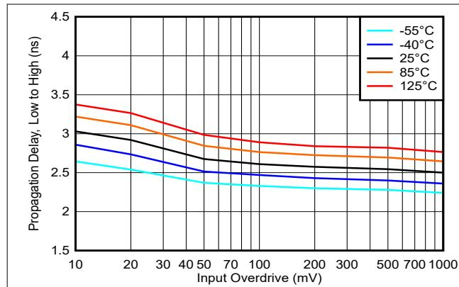
図 5-27. Propagation Delay, Low to High, 2.5V
