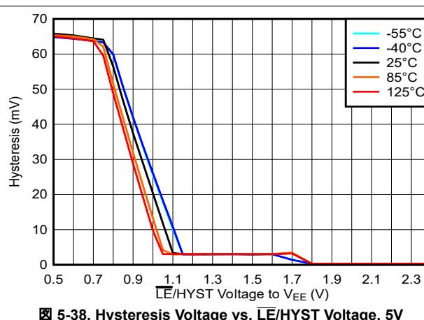
図 5-38. Hysteresis Voltage vs. LE/HYST Voltage, 5V
