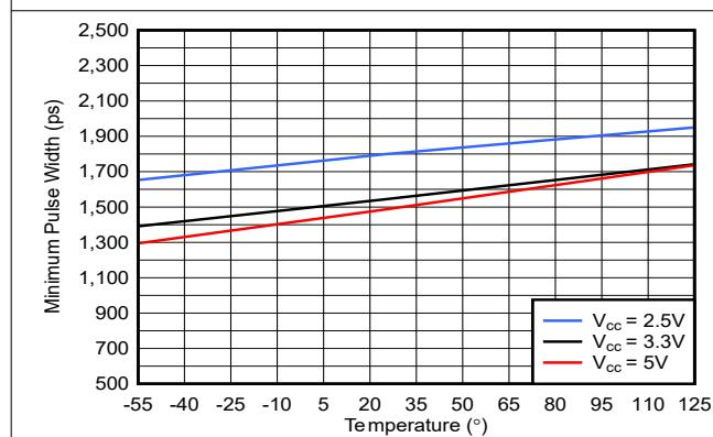
図 5-35. Minimum Pulse Width vs. Temperature
