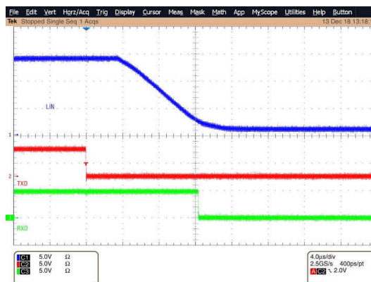
9-12. Recessive to Dominant Propagation Delay
