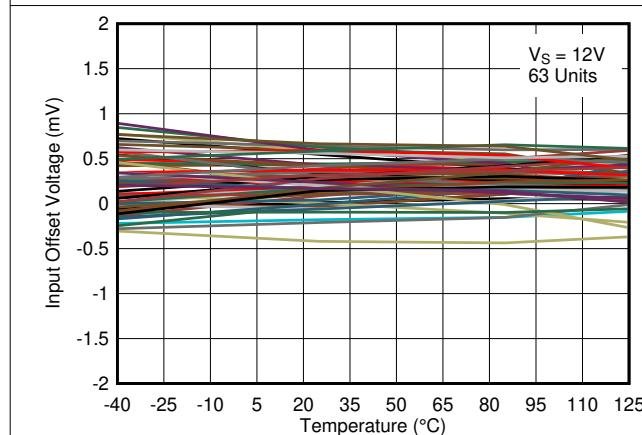
図 5-17. Input Offset Voltage vs. Temperature at 12V
