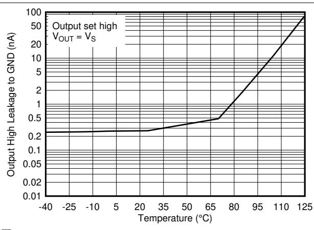
图 5-24. Output High Leakage Current vs. Temperature at 36V
