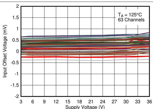
図 5-14. Input Offset Voltage vs. Supply Voltage at  $125^\circ\text{C}$
