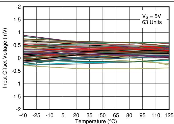
図 5-16. Input Offset Voltage vs. Temperature at 5V
