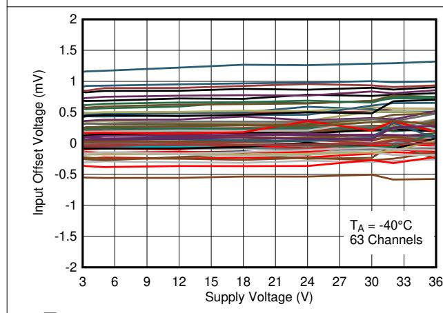
图 5-11. Input Offset Voltage vs. Supply Voltage at -40°C
