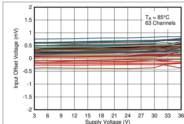
図 5-13. Input Offset Voltage vs. Supply Voltage at  $85^\circ\text{C}$
