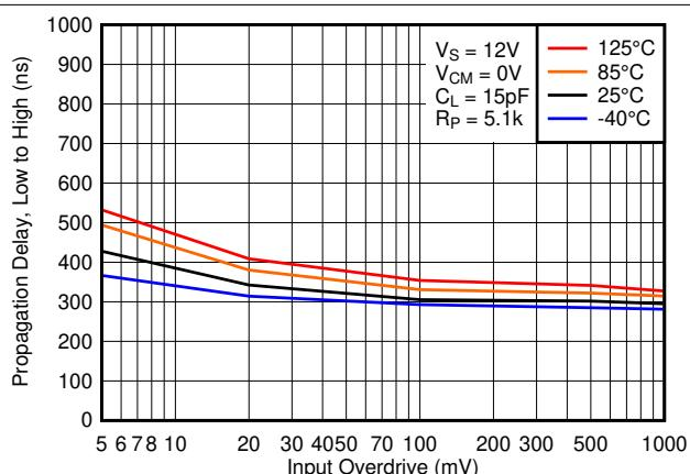
图 5-28. Low to High Propagation Delay vs. Input Overdrive Voltage, 12V
