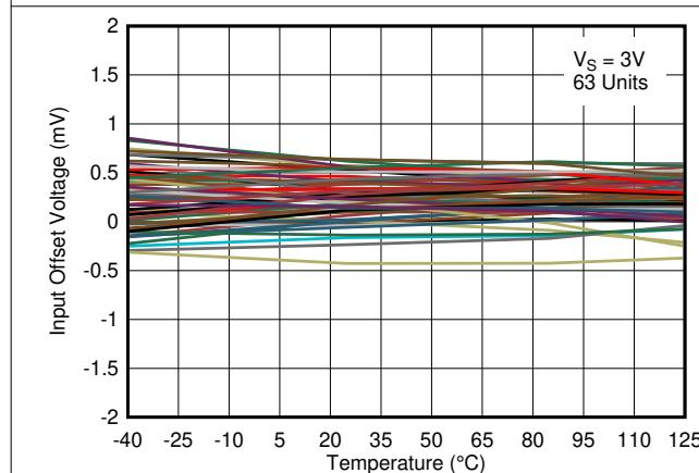
図 5-15. Input Offset Voltage vs. Temperature at 3V
