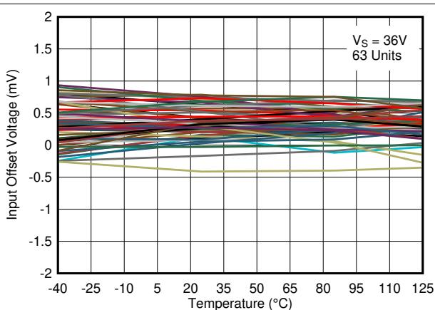
図 5-18. Input Offset Voltage vs. Temperature at 36V
