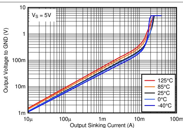
图 5-20. Output Low Voltage vs. Output Sinking Current at 5V
