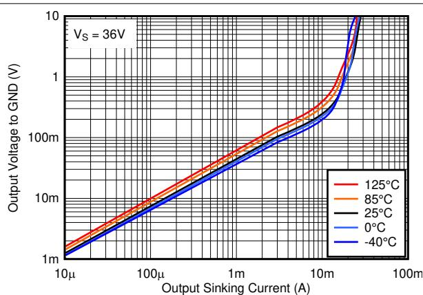
图 5-22. Output Low Voltage vs. Output Sinking Current at 36V
