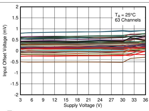
图 5-12. Input Offset Voltage vs. Supply Voltage at 25°C
