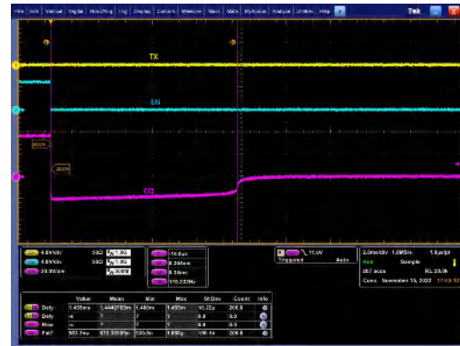
9-5. CQ in Current Fault Auto Recovery, High Side Mode
