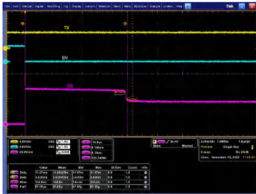
9-4. CQ in Current Fault Auto Recovery, Low Side Mode
