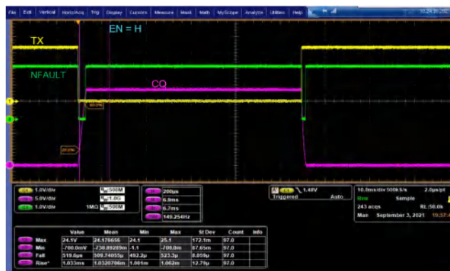
9-6. CQ Driving Inductive Load, Low Side Mode (NPN mode)
