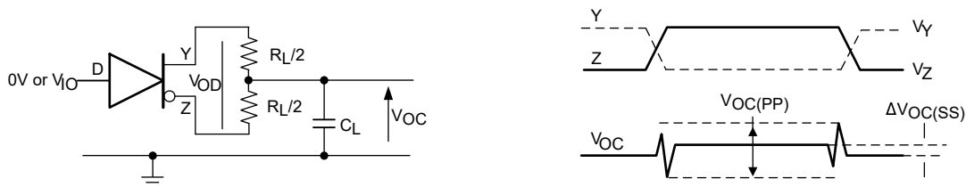
图 6-2. Measurement of Driver Differential and Common-Mode Output With RS-485 Load
