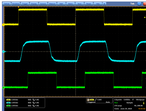
Ch 1: D Input, Ch2: V_A Ch3: V_B Ch4: R V_{CC} = 3.3V Output Data rate: 20Mbps
