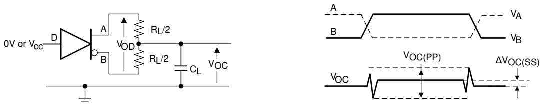
图 8. Measurement of Driver Differential and Common-Mode Output With RS-485 Load
