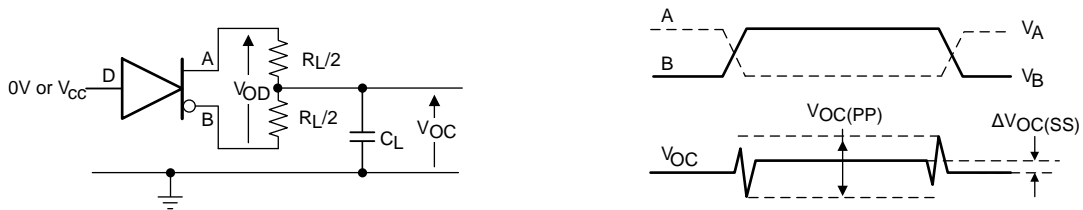
图 9. Measurement of Driver Differential and Common-Mode Output With RS-485 Load
