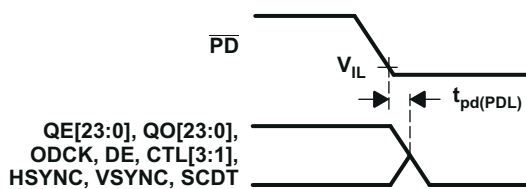
图 6-6. Delay From \overline{PD} Low to Hi-Z Outputs
