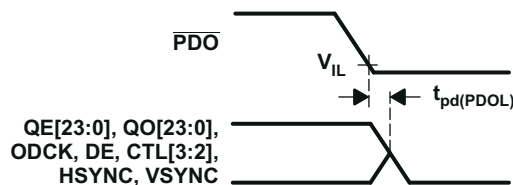
8-8. Delay From \overline{\text{PDO}} Low to Hi-Z Outputs
