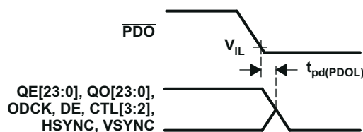
8-8. Delay From \overline{\text{PDO}} Low to Hi-Z Outputs
