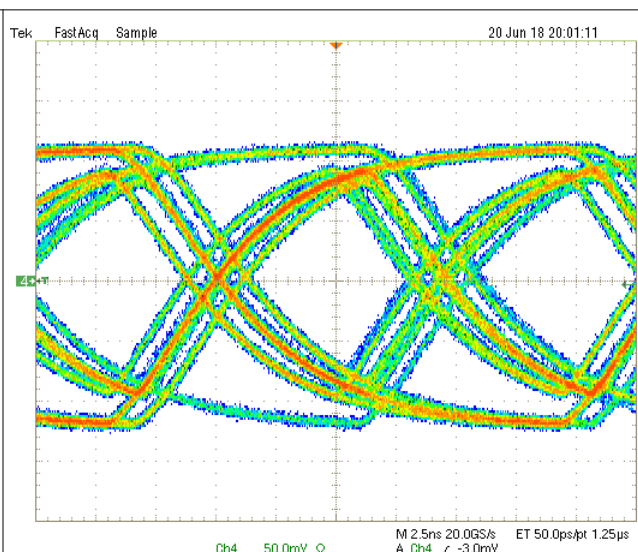
6-12. Back Channel Output Typical Waveform
