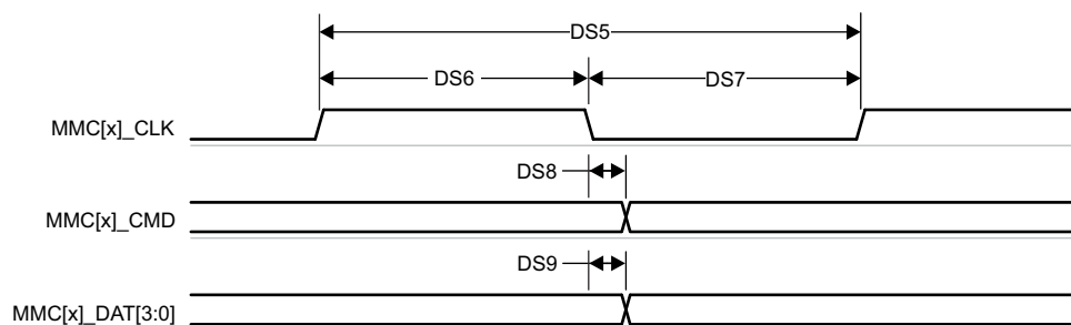
図 6-98. MMC1/2 – Default Speed – Transmit Mode
