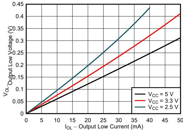
图 6-3. Typical ( $T_A=25^\circ\text{C}$ ) Output Low Voltage ( $V_{\text{OL}}$ ) vs Sink Current ( $I_{\text{OL}}$ )
