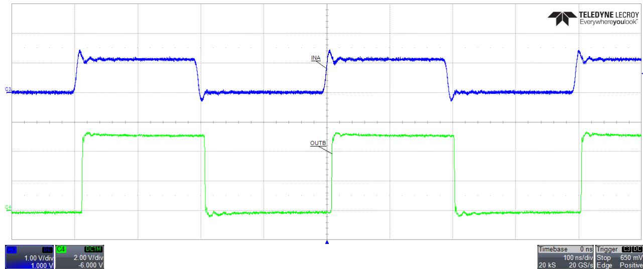
图 9-2. Up Translation at 2.5 MHz (1.2 V to 5 V)
