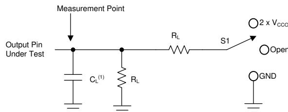
A.  $C_L$  includes probe and jig capacitance.
