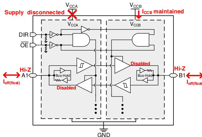
FIG 8-2.  $V_{CC}$  Disconnect Feature
