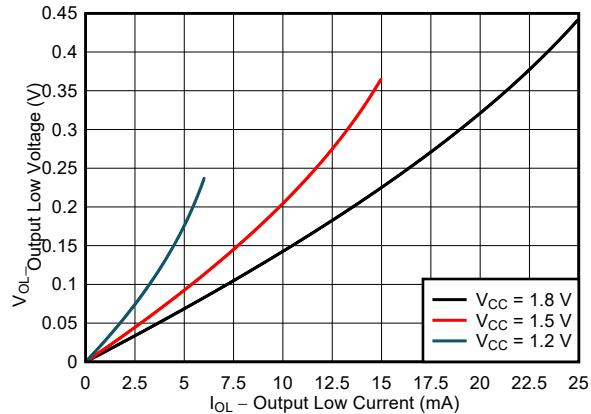
图 6-4. Typical ( $T_A=25^\circ\text{C}$ ) Output Low Voltage ( $V_{\text{OL}}$ ) vs Sink Current ( $I_{\text{OL}}$ )
