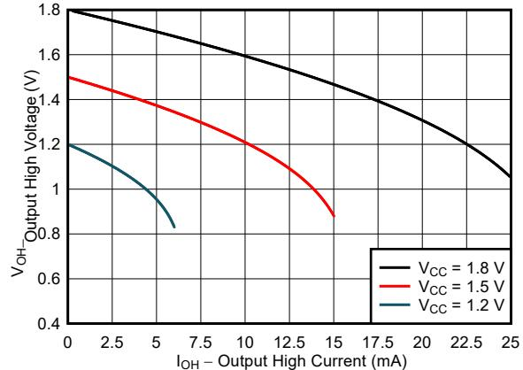
图 6-2. Typical ( $T_A=25^\circ\text{C}$ ) Output High Voltage ( $V_{\text{OH}}$ ) vs Source Current ( $I_{\text{OH}}$ )
