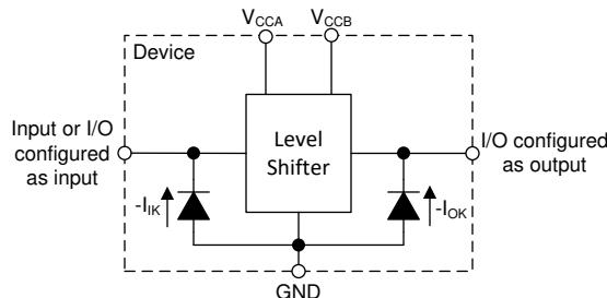
**図 8-3. Electrical Placement of Clamping Diodes for Each Input and Output**
