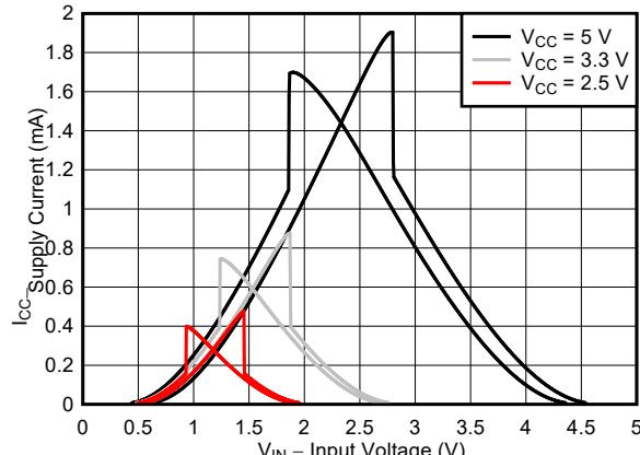
图 6-5. Typical ( $T_A=25^\circ\text{C}$ ) Supply Current ( $I_{\text{CC}}$ ) vs Input Voltage ( $V_{\text{IN}}$ )
