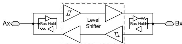
**图 8-4. Schematic Description of Location of Bus-Hold Circuits**
