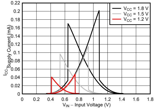
图 6-6. Typical ( $T_A=25^\circ\text{C}$ ) Supply Current ( $I_{\text{CC}}$ ) vs Input Voltage ( $V_{\text{IN}}$ )
