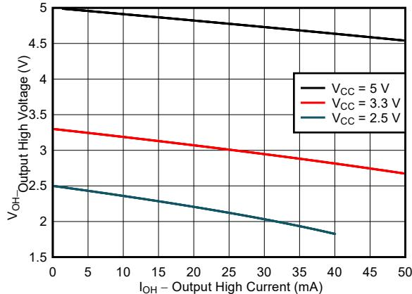
图 6-1. Typical ( $T_A=25^\circ\text{C}$ ) Output High Voltage ( $V_{\text{OH}}$ ) vs Source Current ( $I_{\text{OH}}$ )
