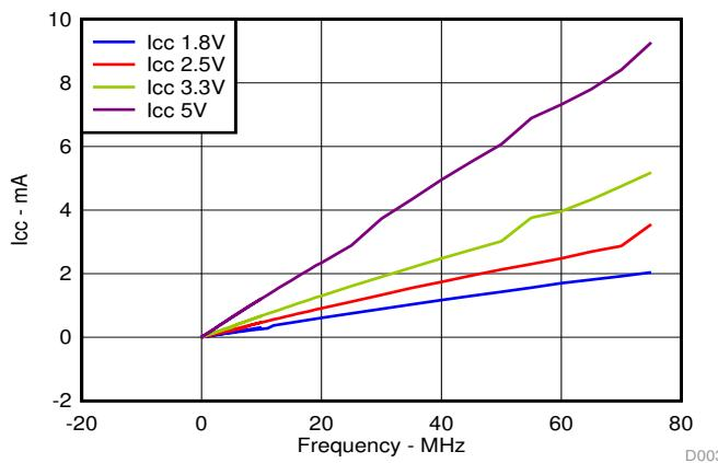
**Figure 6. I<sub>CC</sub> vs Frequency**
