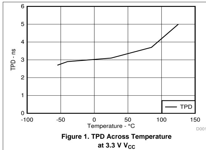
**Figure 1.** TPD Across Temperature at 3.3 V  $V_{CC}$
