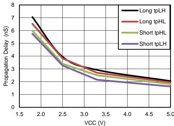
(1) Short is 2 inverter path. Long is 3 inverter path.
