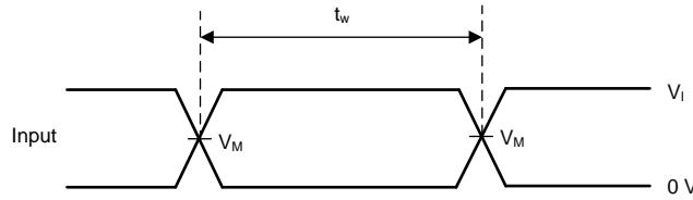
**図 3. Voltage Waveforms: Pulse Duration**
