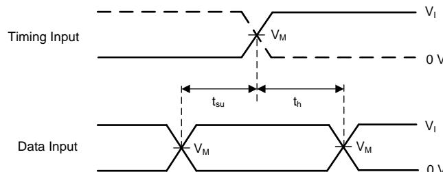
**図 5. Voltage Waveforms: Setup and Hold Times**
