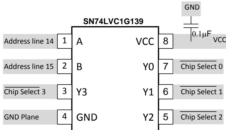
図 7. Typical Application Diagram
