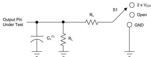
(1)  $C_L$  includes probe and jig capacitance.
