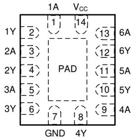
図 5-1. SN74LV6T06 BQA Package, 14-Pin WQFN (Top View)
