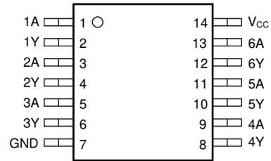
図 5-2. SN74LV6T06 PW Package, 14-Pin TSSOP (Top View)
