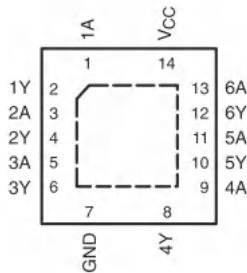
**图 5-2. SN74LV14A RGY Package Top View**
