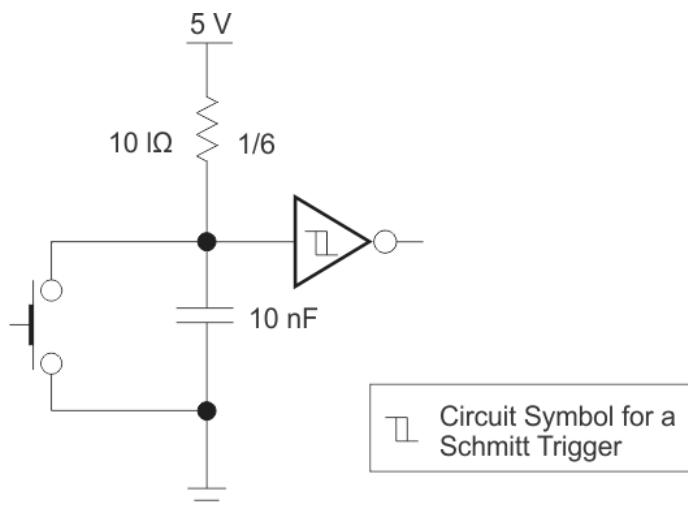
図 9-2. Switch De-bouncer Schematic
