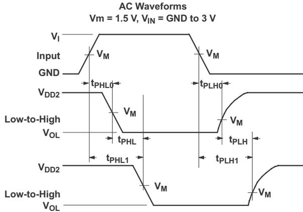
図 7-1. Input (Sn) to Output (Dn) Propagation Delays
