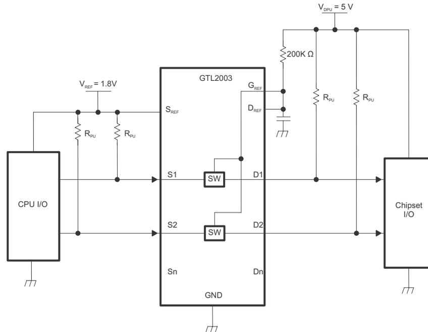
図 9-4. Unidirectional Up Translation to Higher-Voltage Chipsets
