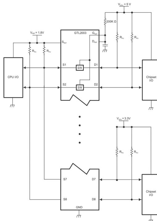
**図 9-1. Bidirectional Translation to Multiple Higher Voltage Levels (Such as an I<sup>2</sup>C or SMBus Applications)**
