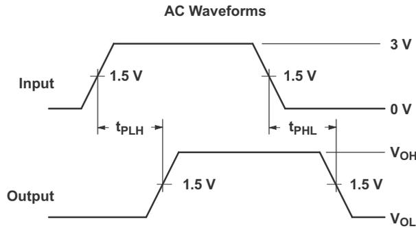
図 7-3. Input (Sn) to Output (Dn) Propagation Delays
