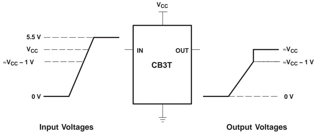
NOTE A: If the input high voltage ( $V_{IH}$ ) level is greater than or equal to  $V_{CC} - 1\text{ V}$ , and less than or equal to 5.5 V, then the output high voltage ( $V_{OH}$ ) level will be equal to approximately the  $V_{CC}$  voltage level.
