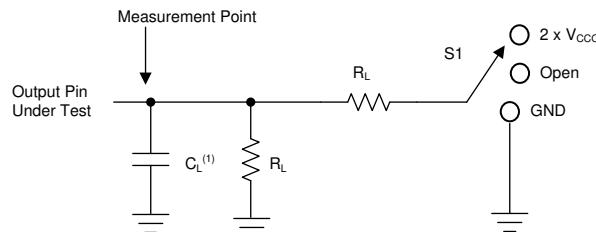
A.  $C_L$  includes probe and jig capacitance.
