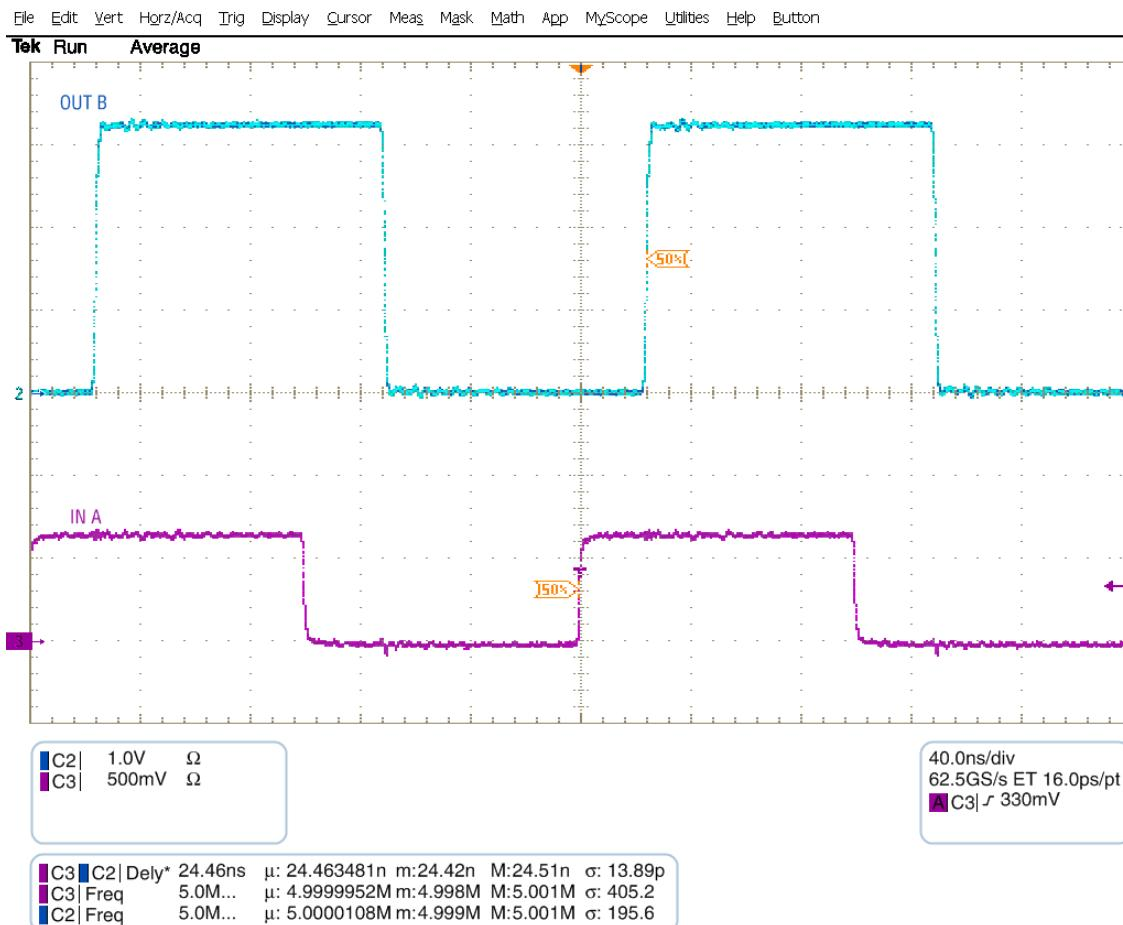
図 8-2. Up Translation at 2.5 MHz (0.7V to 3.3V)
