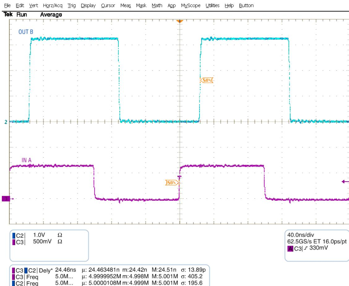
図 8-4. Up Translation at 2.5 MHz (0.7V to 3.3V)
