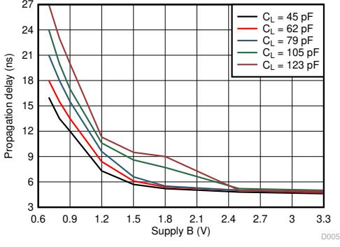
$T_A = 25^\circ\text{C}$     $V_{CCA} = 1.8\text{V}$
