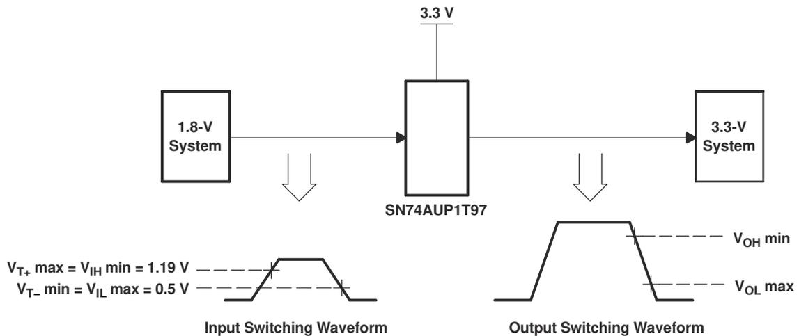
7-3. Switching Thresholds for 1.8-V to 3.3-V Translation
