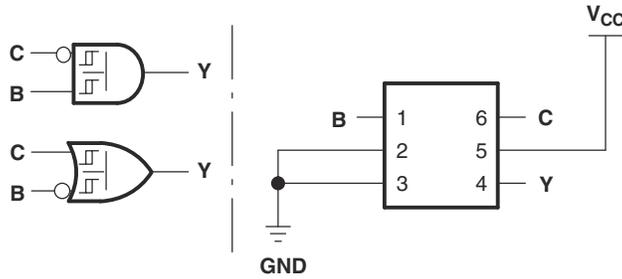
7-7. 14+08/14+02: 2-Input AND/NOR Gate With One Inverted Input
