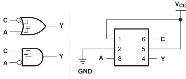
7-6. 14+32/14+00: 2-Input OR/NAND Gate With One Inverted Input
