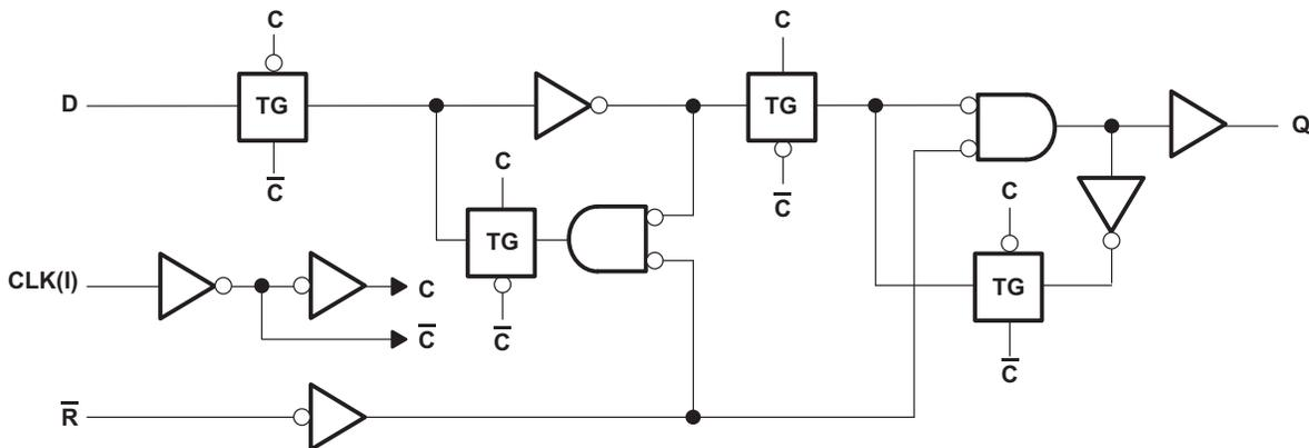
图 7-2. Logic Diagram, Each Flip-flop (Positive Logic)
