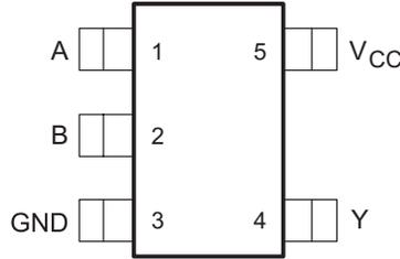
☒ 4-1. DBV Package 5-Pin SOT-23 Top View
