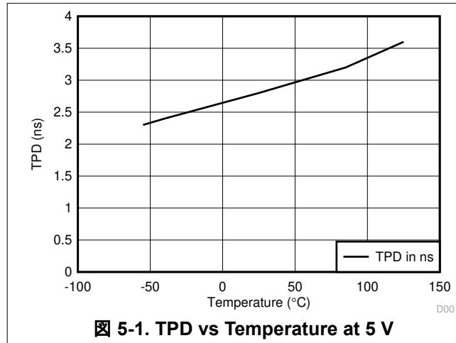
図 5-1. TPD vs Temperature at 5 V
