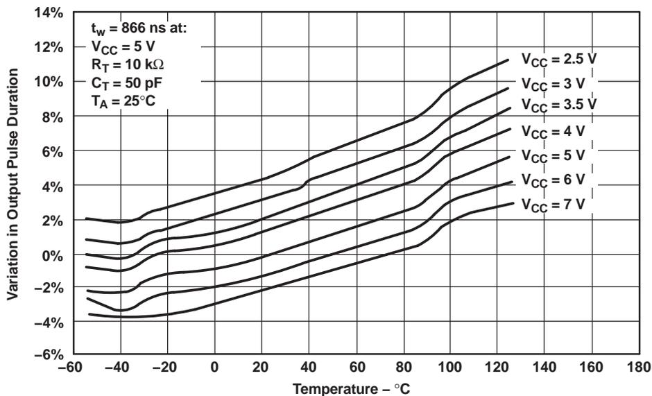
Figure 6. Variations in Output Pulse Duration vs Temperature
