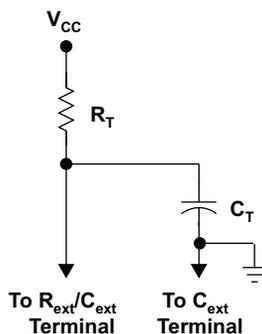
Figure 2. Timing-Component Connections
