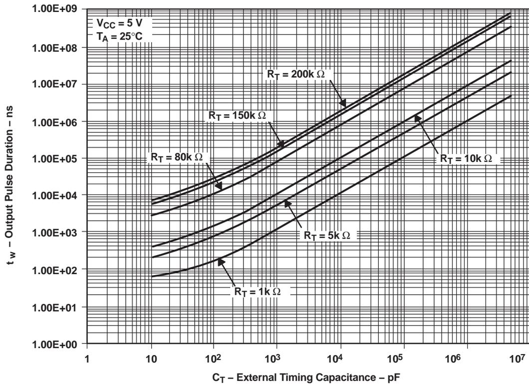
Figure 5. Output Pulse Duration vs External Timing Capacitance
