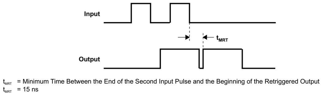
Figure 4. Input/Output Requirements
