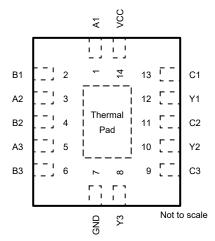
Figure 4-1. SN74AC3G97-Q1 PW Package (Preview), 14-Pin TSSOP (Top View)
