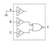
2-Input NOR with 1 inverted input
