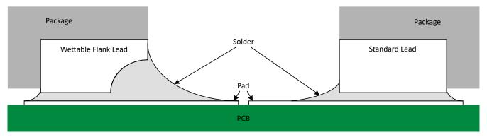
Figure 7-1. Simplified Cutaway View of Wettable-Flank QFN Package and Standard QFN Package After Soldering
