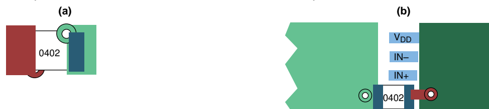
Figure 28. Typical Decoupling Capacitor Layouts
