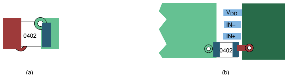
Figure 33. Typical Decoupling Capacitor Layouts
