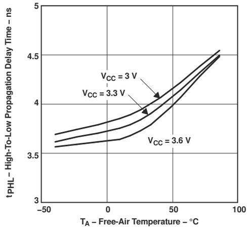
**5-4. High-to-Low Propagation Delay Time vs Free-Air Temperature**
