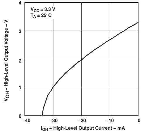
**5-2. High-Level Output Voltage vs High-Level Output Current**
