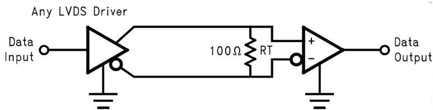
Figure 7-1. Application Diagram
