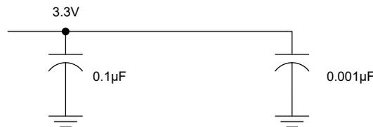
图 9-1. Recommended LVDS Bypass Capacitor Layout
