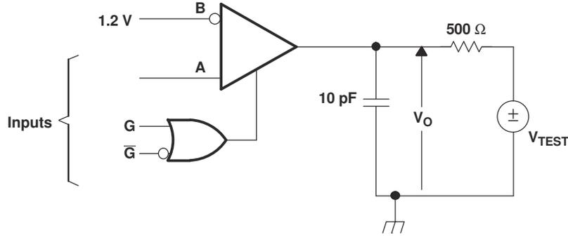
NOTE: All input pulses are supplied by a generator having the following characteristics:  $t_r$  or  $t_f \leq 1$  ns, pulse repetition rate (PRR) = 0.5 Mpps, pulsewidth =  $500 \pm 10$  ns.  $C_L$  includes instrumentation and fixture capacitance within 0,06 mm of the D.U.T.
