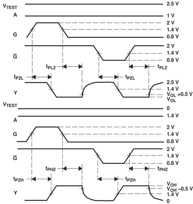
図 6-4. Enable/Disable Time Test Circuit and Waveforms
