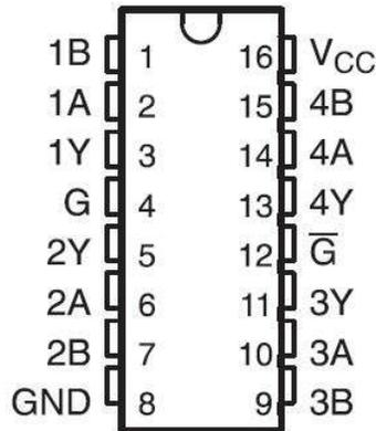
☒ 4-1. D Package 16-Pin, SOIC (Top View)
