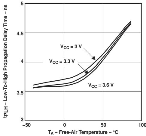
**5-3. Low-to-High Propagation Delay Time vs Free-Air Temperature**
