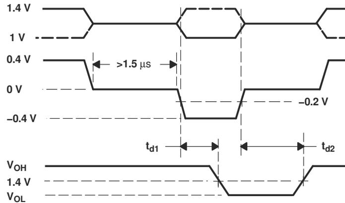
☒ 6-6. Waveforms for Failsafe Activate and Deactivate
