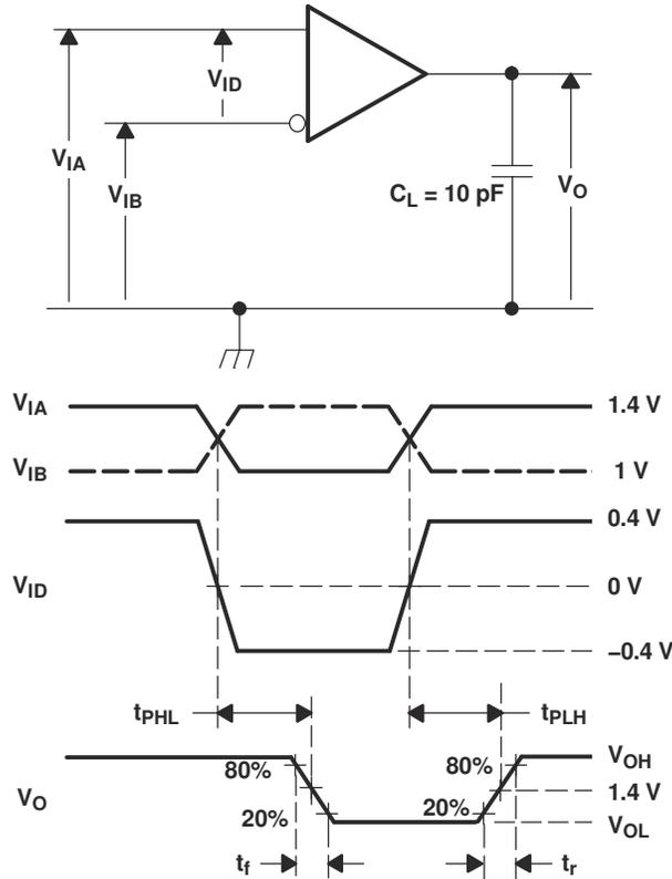
All input pulses are supplied by a generator having the following characteristics:  $t_r$  or  $t_f \leq 1\text{ns}$ , pulse repetition rate (PRR) = 50Mpps [pps : pulse per second], pulse width =  $10 \pm 0.2\text{ns}$ .  $C_L$  includes instrumentation and fixture capacitance within 0,06mm of the D.U.T.
