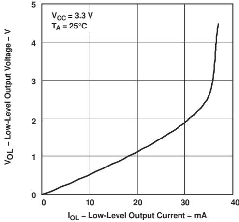
**5-1. Low-Level Output Voltage vs Low-Level Output Current**
