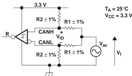
The R Output State Does Not Change During Application of the Input Waveform.
