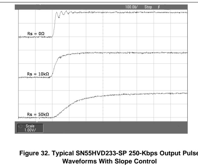
**Figure 32. Typical SN55HVD233-SP 250-Kbps Output Pulse Waveforms With Slope Control**
