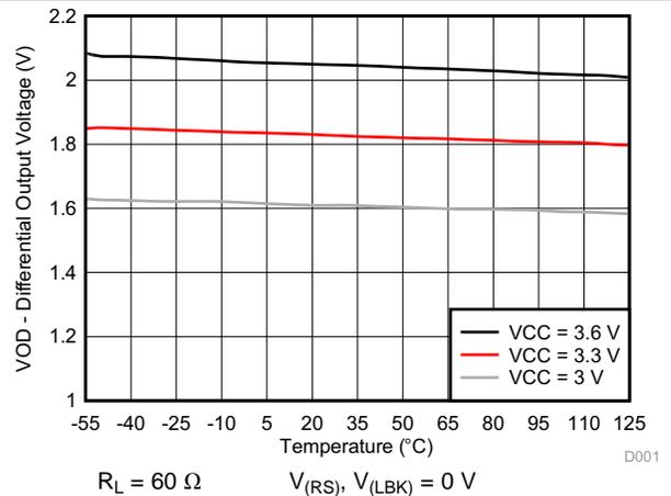
Figure 6. Differential Output Voltage vs Temperature
