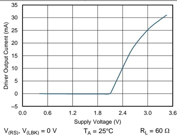
Figure 11. Driver Output Current vs Supply Voltage
