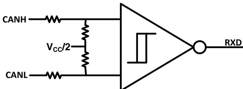
Figure 26. Simplified Recessive Common Mode Bias and Receiver
