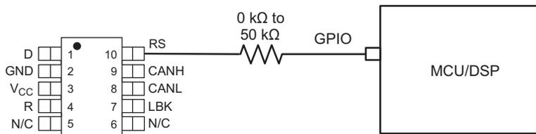
**Figure 30. Slope Control/Standby Connection to a DSP**
