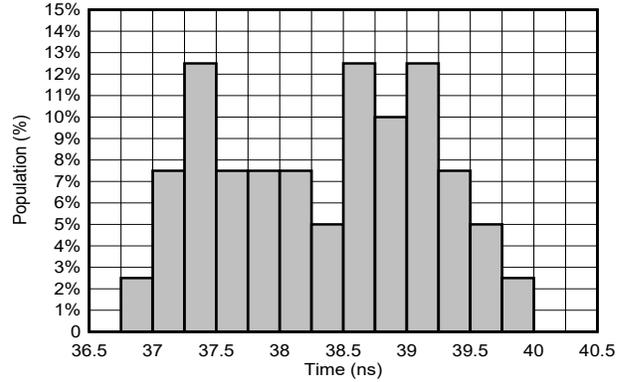
6-14.  $T_{PD}$  Distribution; 1.2-V;  $T_A = -55^\circ\text{C}$  to  $125^\circ\text{C}$  (40 Samples)
