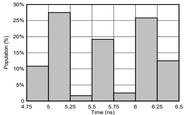
6-18.  $T_{PD}$  Distribution; 5-V;  $T_A = -55^\circ\text{C}$  to  $125^\circ\text{C}$  (40 Samples)
