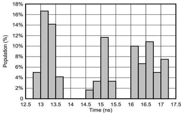
6-15.  $T_{PD}$  Distribution; 1.8-V;  $T_A = -55^\circ\text{C}$  to  $125^\circ\text{C}$  (40 Samples)
