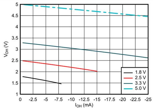
6-4. Output Voltage vs Current in HIGH State
