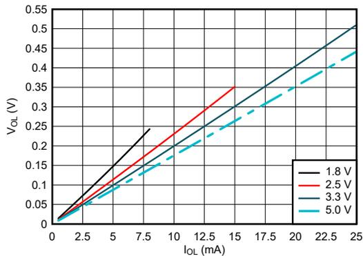
6-5. Output Voltage vs Current in LOW State
