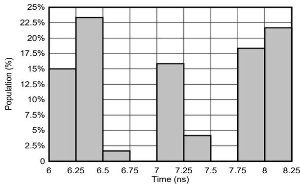
6-17.  $T_{PD}$  Distribution; 3.3-V;  $T_A = -55^\circ\text{C}$  to  $125^\circ\text{C}$  (40 Samples)
