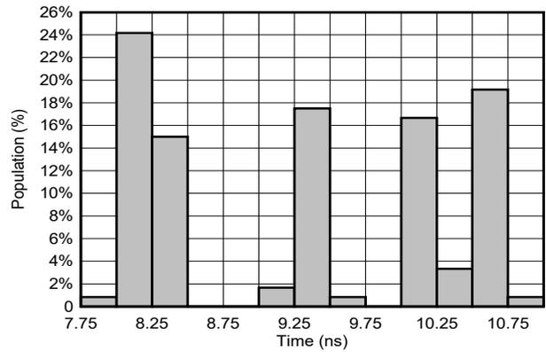
6-16.  $T_{PD}$  Distribution; 2.5-V;  $T_A = -55^\circ\text{C}$  to  $125^\circ\text{C}$  (40 Samples)
