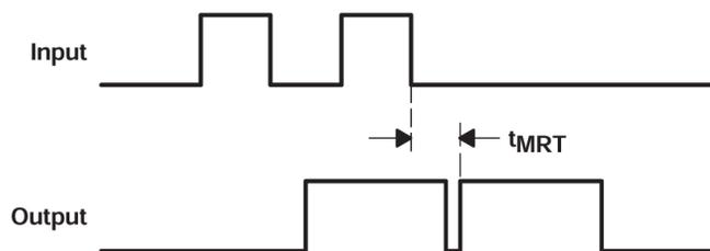
$t_{MRT}$  = Minimum Time Between the End of the Second Input Pulse and the Beginning of the Retriggered Output
