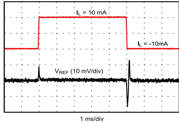
図 6-38. 負荷過渡応答 ( $C_{OUT} = 10\mu\text{F}$ )
