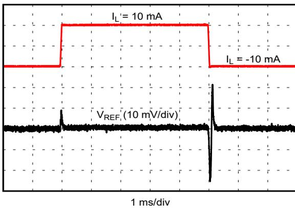
図 6-39. 負荷過渡応答 ( $C_{OUT} = 1\mu\text{F}$ )
