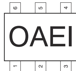
✎ 5-2. DBV Package, 6-Pin SOT-23 (Top View)
