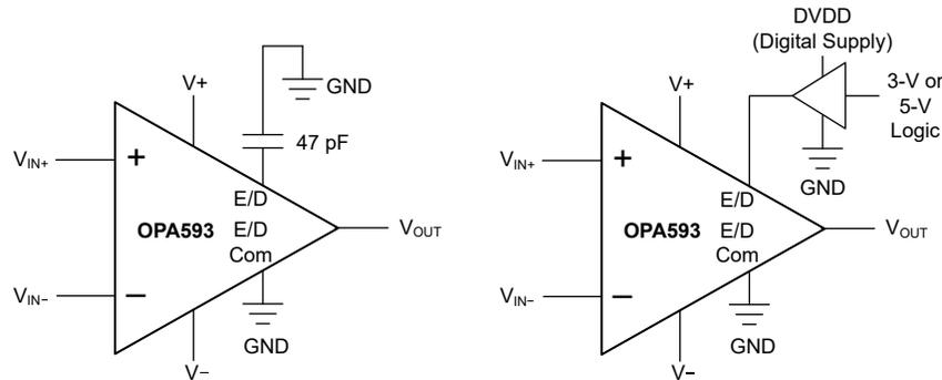
**Figure 7-3. E/D and E/D Com Pin Connections**
