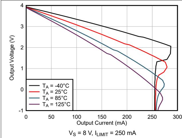
Fig 6-25. Output Voltage vs Output Sourcing Current
