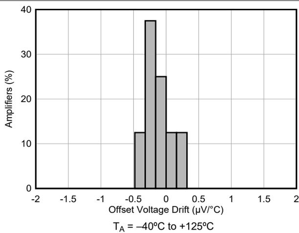
6-5. Input Offset Voltage Drift Distribution
