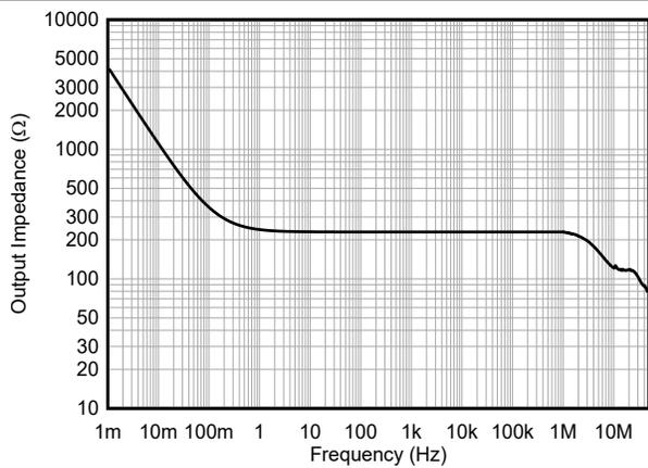
6-41. Open-Loop Output Impedance vs Frequency
