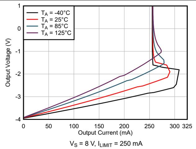
Fig 6-26. Output Voltage vs Output Sinking Current
