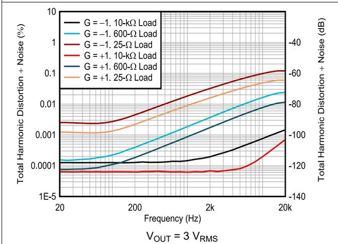
6-45. Total Harmonic Distortion + Noise vs Frequency
