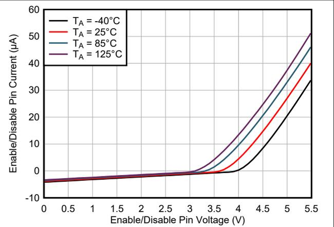
6-70. Enable Pin Current vs Enable Pin Voltage
