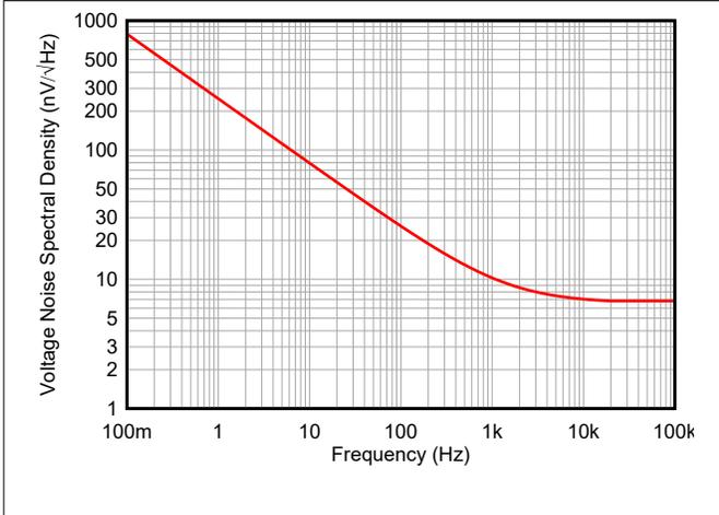
6-43. Input Voltage Noise Spectral Density
