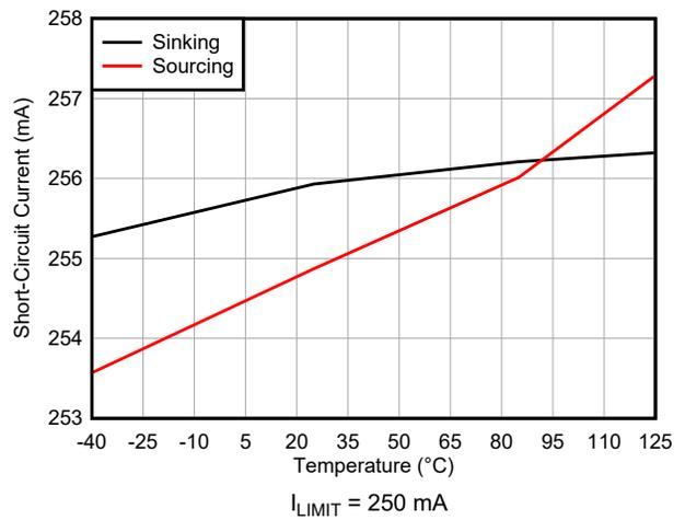
6-40. Short Circuit Current vs Temperature
