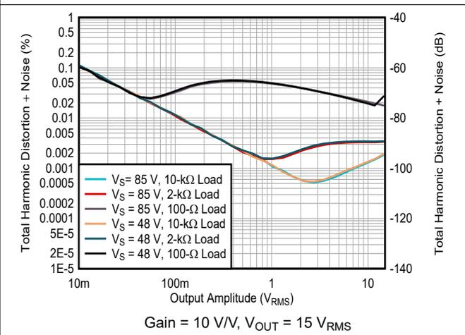
6-48. Total Harmonic Distortion + Noise vs Amplitude
