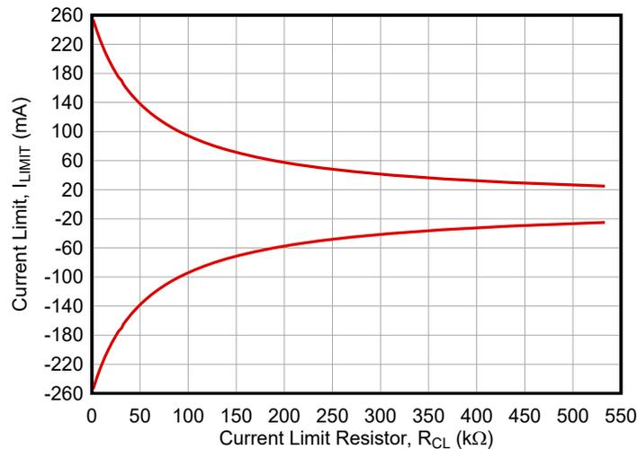
**Figure 7-2. Typical Output Current vs Current-Limit Resistor Value**
