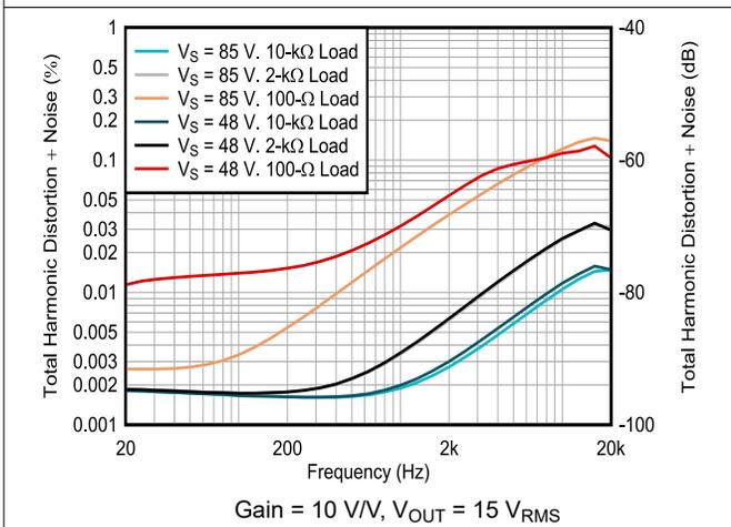
6-47. Total Harmonic Distortion + Noise vs Frequency
