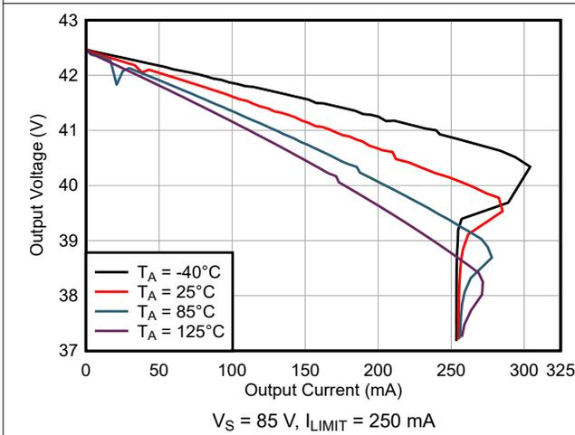
Fig 6-29. Output Voltage vs Output Sourcing Current
