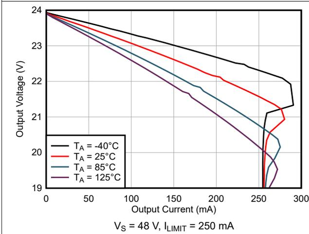
Fig 6-27. Output Voltage vs Output Sourcing Current
