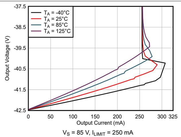
Fig 6-30. Output Voltage vs Output Sinking Current
