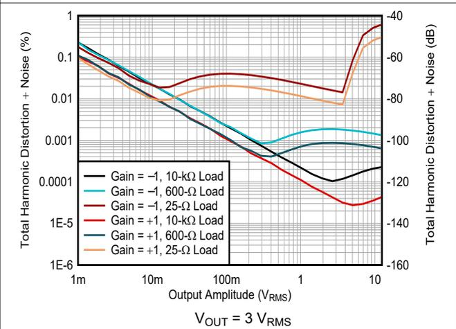
6-46. Total Harmonic Distortion + Noise vs Amplitude
