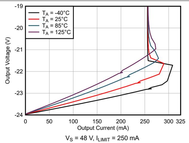
Fig 6-28. Output Voltage vs Output Sinking Current
