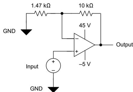
图 8-1. Output Driver Configured With a Gain of 8
