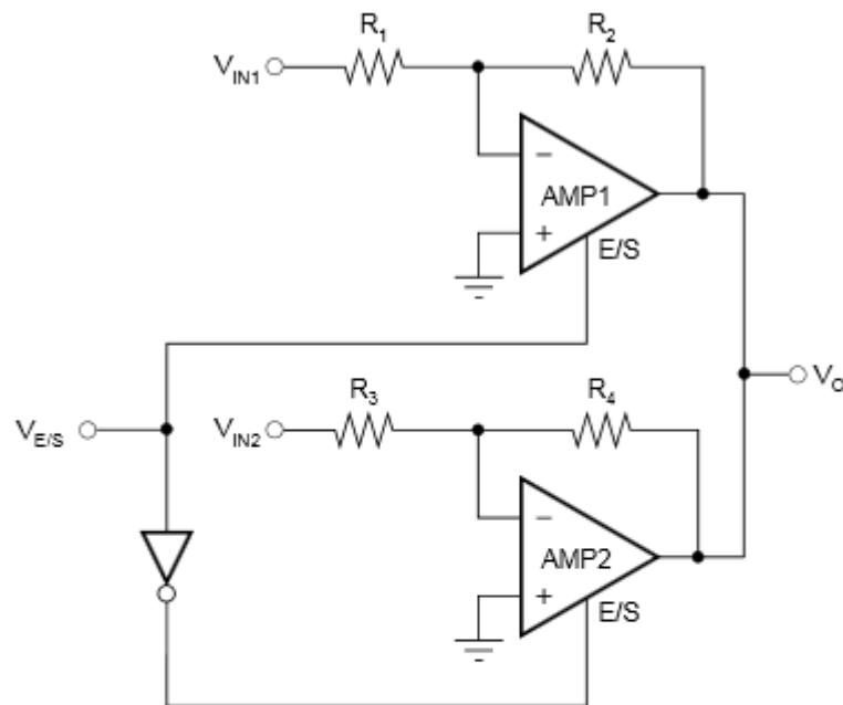
$V_{E/S} > (V-) + 2.4V$ : Amp 1 is on, Amp 2 if off
