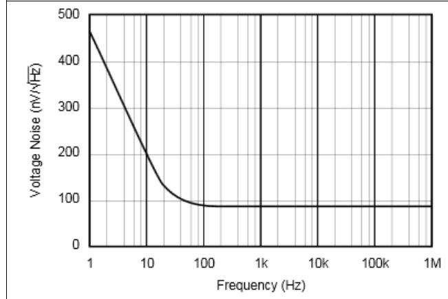
**Figure 9. Voltage Noise Density vs Frequency**
