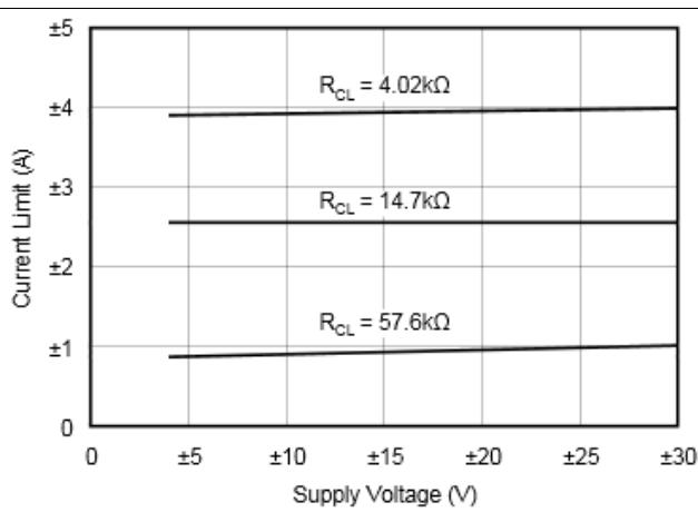
**Figure 4. Current Limit vs Supply Voltage**
