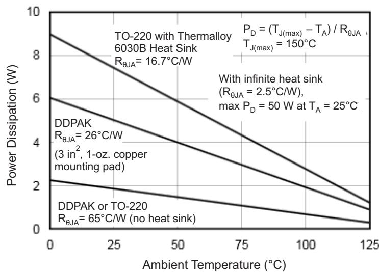
**Figure 44. Maximum Power Dissipation vs Ambient Temperature**
