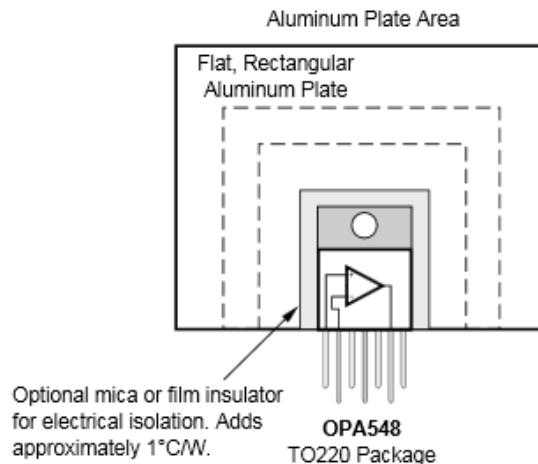
**Figure 42. TO-220 Thermal Resistance vs Aluminum Plate Area**
