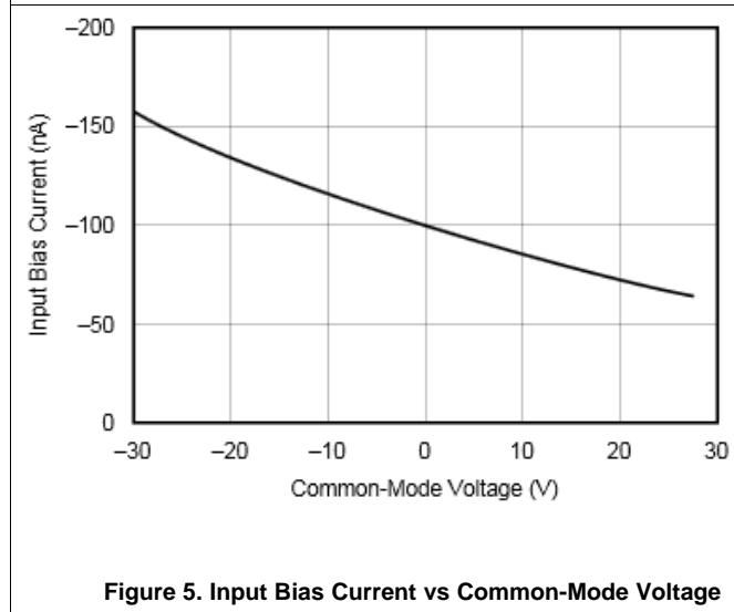
**Figure 5. Input Bias Current vs Common-Mode Voltage**
