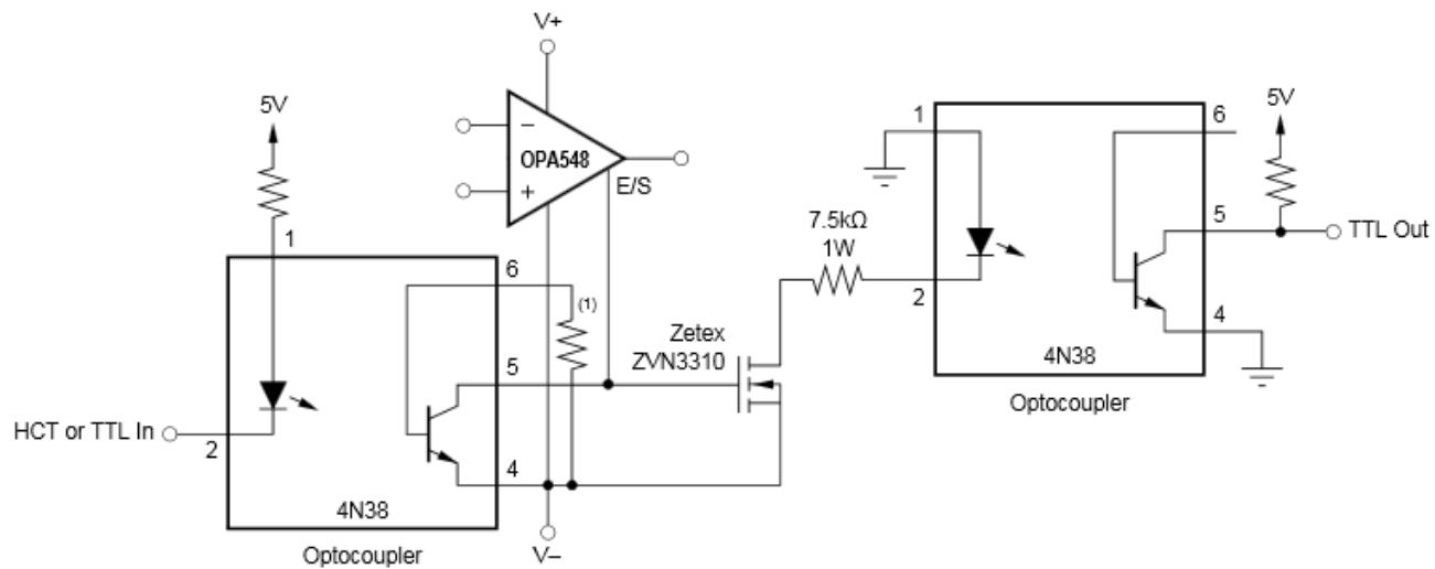
NOTE: (1) Optional—may be required to limit leakage current of optocoupler at high temperatures.
