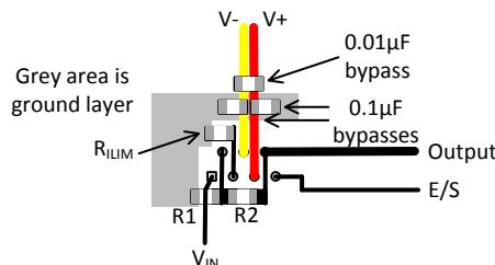
**Figure 45. Recommended Layout Example**
