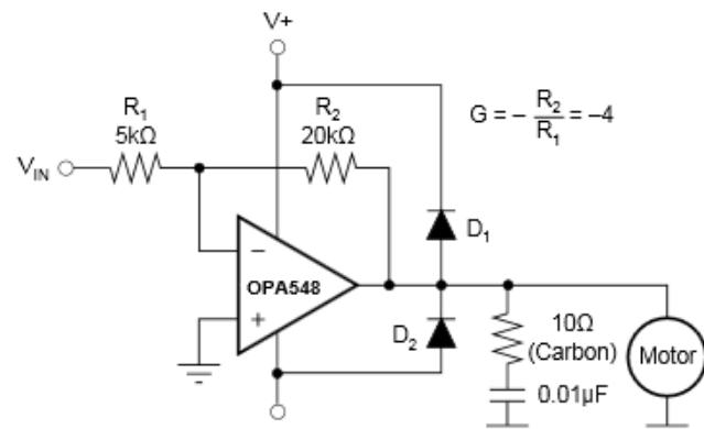
**Figure 38.** Motor Drive Circuit
