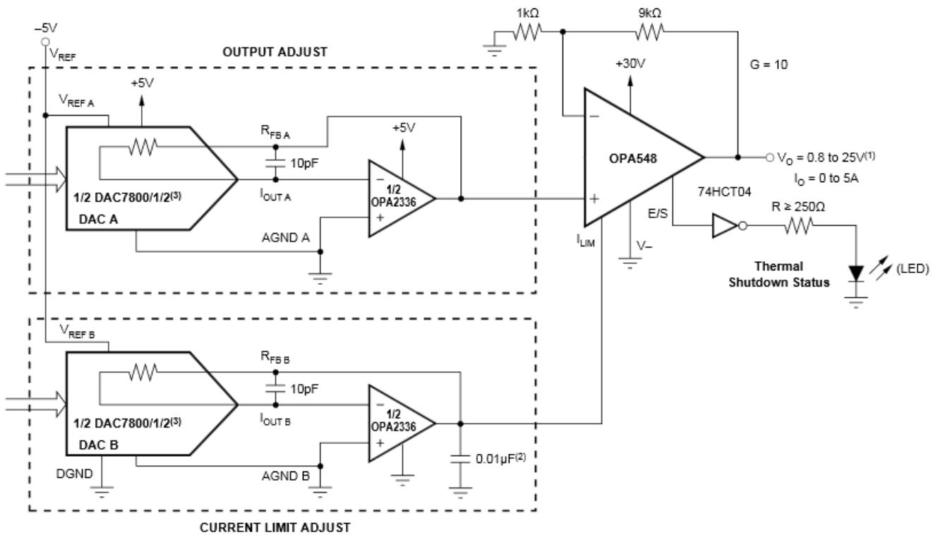
**Figure 32. Digitally-Controlled Programmable Power Supply Schematic**
