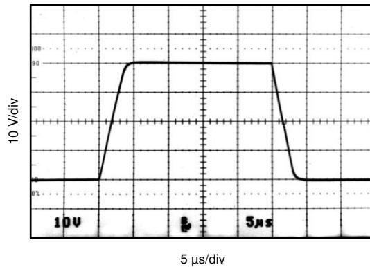
$G = 3$        $C_L = 1000 \text{ pF}$        $R_L = 8 \Omega$
