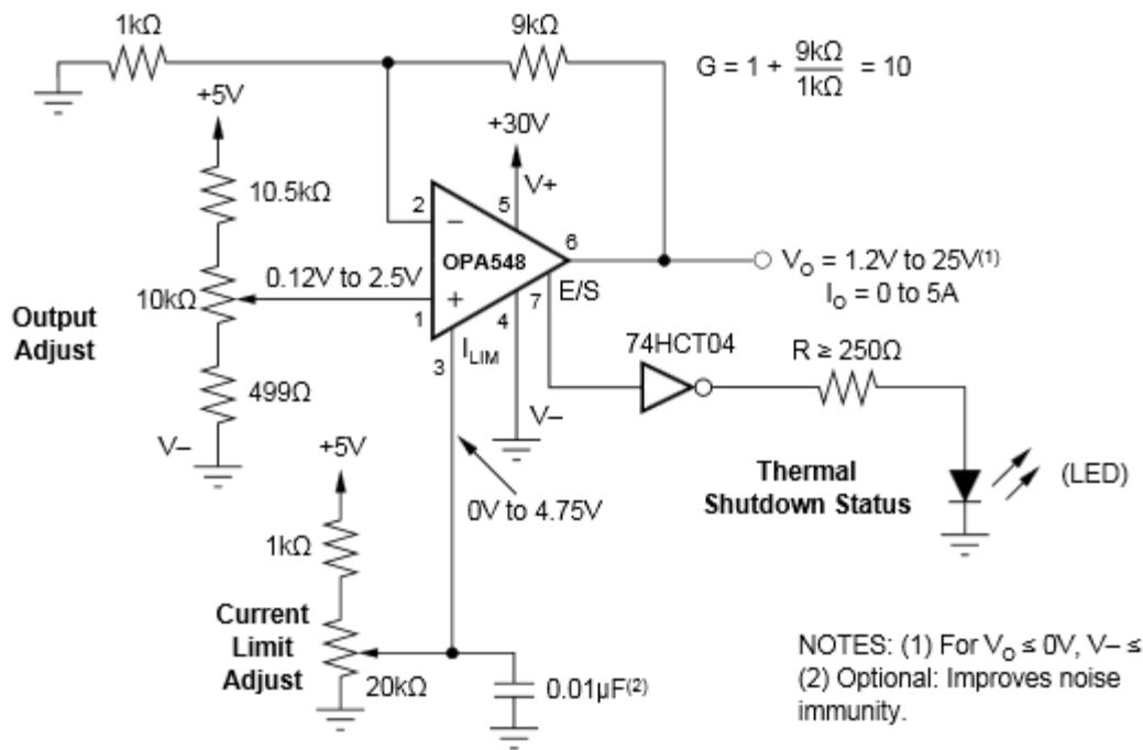
Figure 31. Resistor-Controlled Programmable Power Supply Schematic
