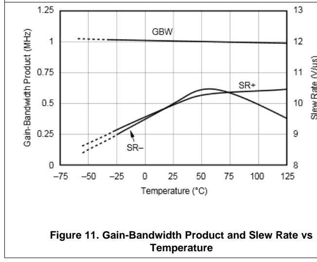
**Figure 11. Gain-Bandwidth Product and Slew Rate vs Temperature**
