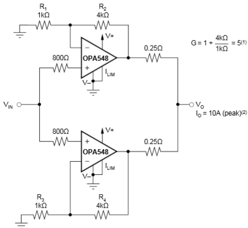
NOTES: (1) Works well for  $G < 10$ . Input offset causes output current to flow between amplifiers with  $G > 10$ . Gains (resistor ratios) of the two amplifiers should be carefully matched to ensure equal current sharing. (2) As configured ( $I_{LIM}$  connected to  $V_-$ ) output current limit is set to 10A (peak). Each amplifier is limited to 5A (peak). Other current limit values may be obtained, see Figure 3, "Adjustable Current Limit".
