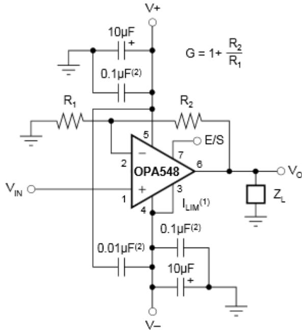
NOTES: (1)  $I_{LIM}$  connected to  $V_-$  gives the maximum current limit, 5A (peak). (2) Connect capacitors directly to package power-supply pins.
