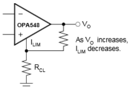
**Figure 35. Single Quadrant  $V \times I$  Limiting**
