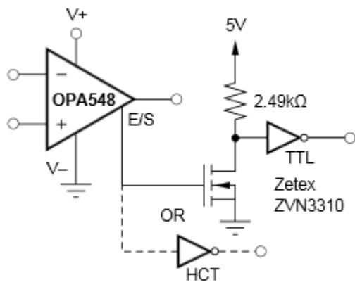
**Figure 28. Thermal Shutdown Status With a Single-Supply**
