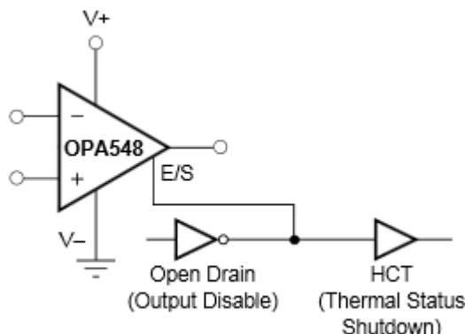
**Figure 37.** Output Disable and Thermal Shutdown Status With a Single Supply
