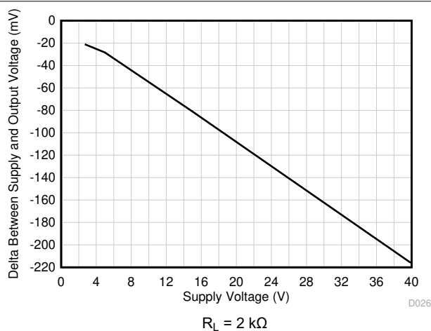
5-30. Output Swing vs Supply Voltage, Negative Swing
