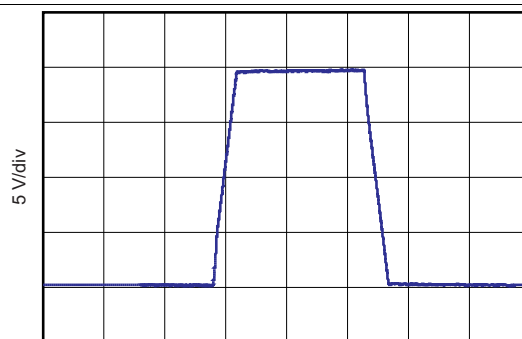
FIG 16. Small-Signal Step Response (100 mV)
