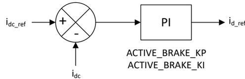
图 7-41. Active Braking Current Control Loop for  $i_{d\_ref}$
