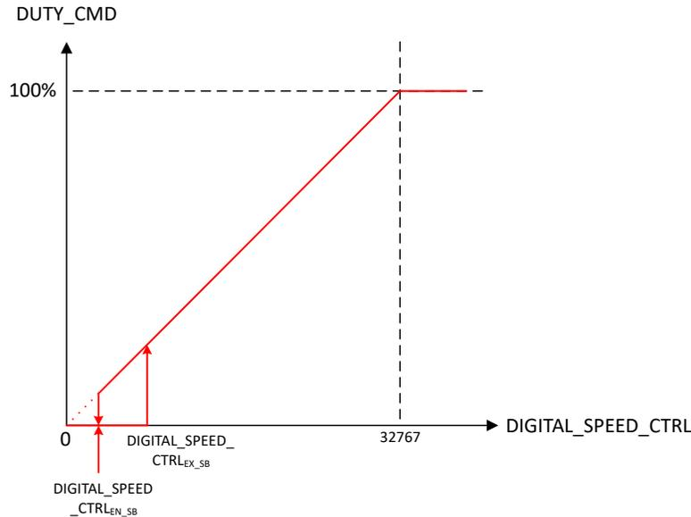
**Figure 7-16. I<sup>2</sup>C-Mode Motor Control**
