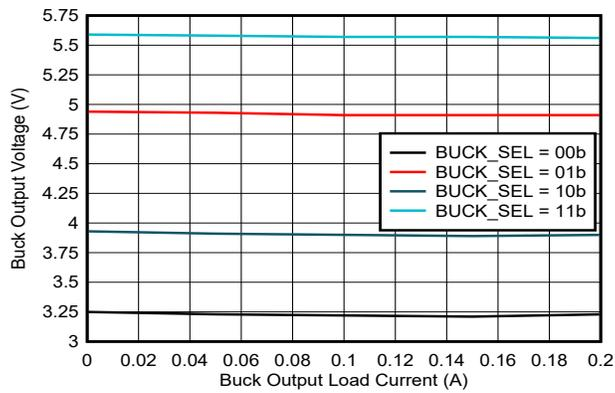
**6-3. Buck regulator output voltage over load current**
