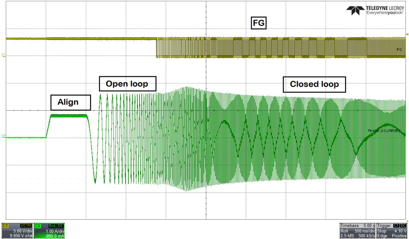
**8-2. Motor Startup - FG and Phase current**
