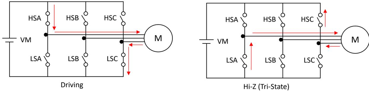
Figure 7-27. IPD Release Mode - Tristate (1b)
