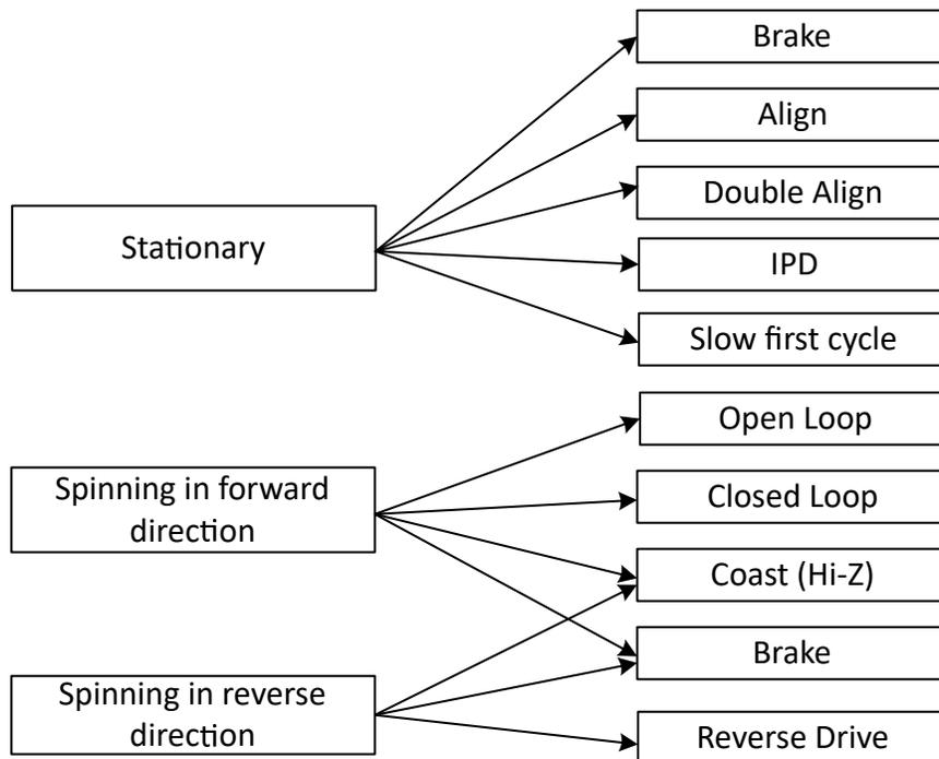
7-21. Starting the motor under different initial conditions
