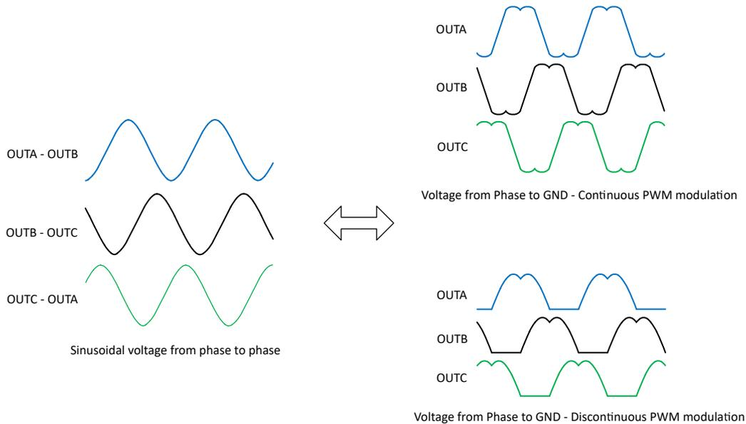
**Figure 7-42. Continuous and Discontinuous PWM Modulation Phase Voltages**
