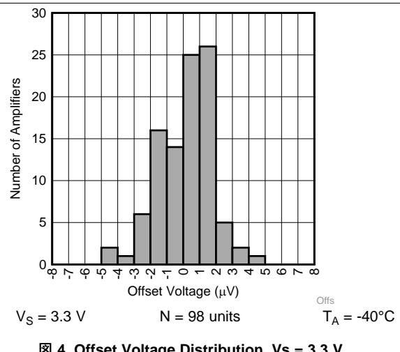
図 4. Offset Voltage Distribution,  $V_S = 3.3\text{ V}$
