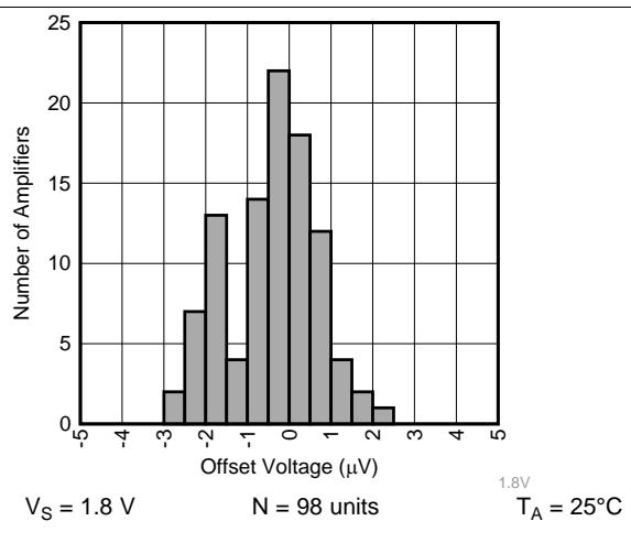
図 2. Offset Voltage Distribution,  $V_S = 1.8\text{ V}$
