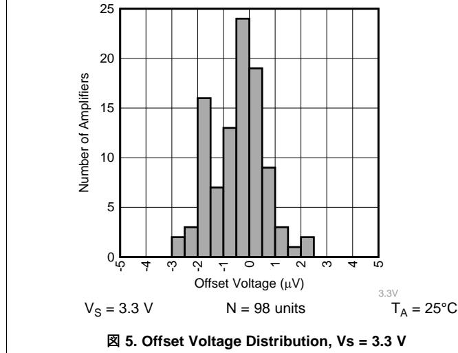
図 5. Offset Voltage Distribution,  $V_S = 3.3\text{ V}$
