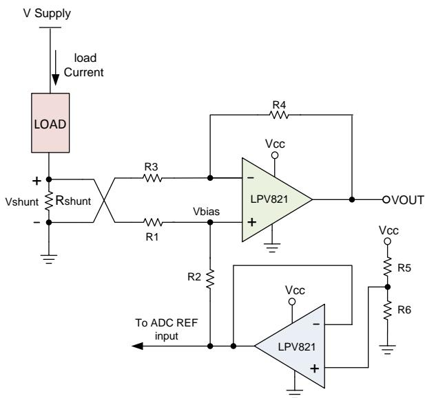
**図 40. Low-Side Current Measurement**
