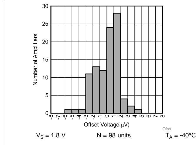
図 1. Offset Voltage Distribution,  $V_S = 1.8\text{ V}$
