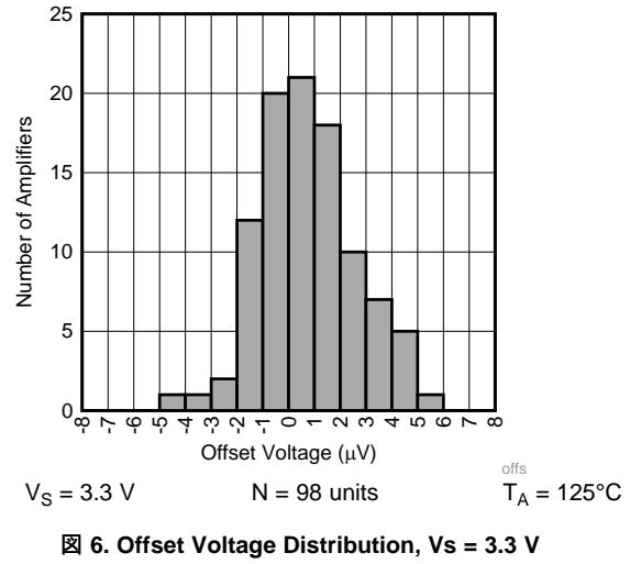
図 6. Offset Voltage Distribution,  $V_S = 3.3\text{ V}$
