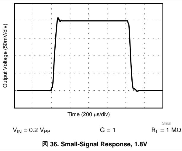
図 36. Small-Signal Response, 1.8V
