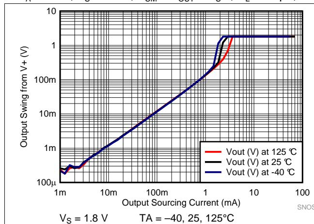
図 31. Output Swing vs Sourcing Current, 1.8 V
