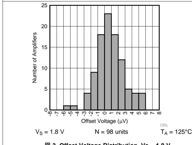
図 3. Offset Voltage Distribution,  $V_S = 1.8\text{ V}$
