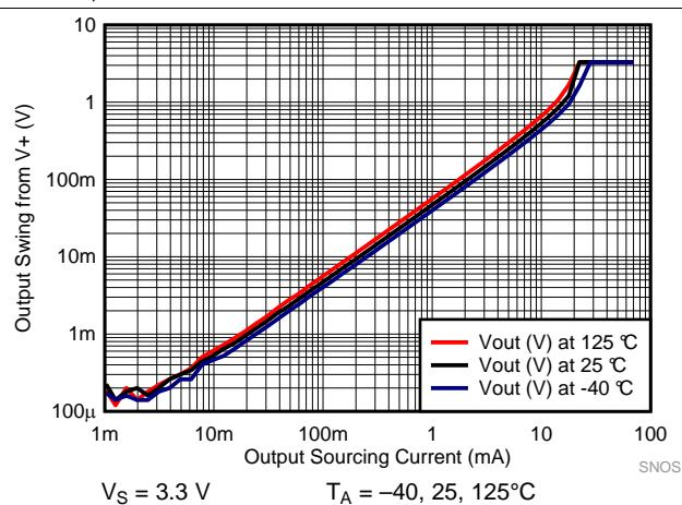
図 32. Output Swing vs Sourcing Current, 3.3 V
