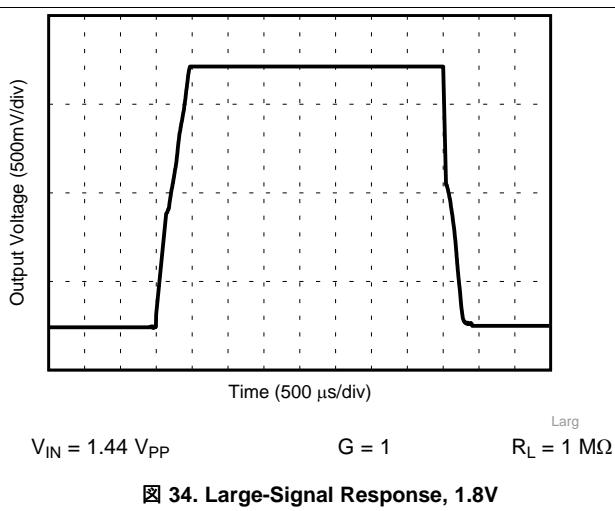
図 34. Large-Signal Response, 1.8V
