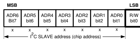
図 6-42. Address and Read/Write Bit
