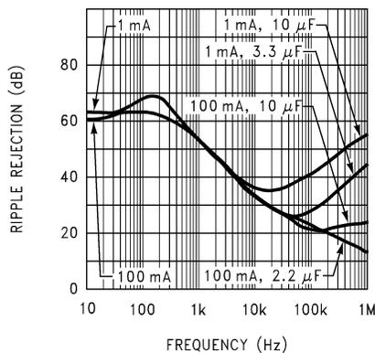
5-41. Ripple Rejection vs Frequency (Legacy Chip)
