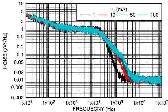
5-45. Output Noise Density vs Load Current ( $I_L$ ) Frequency (New Chip)
