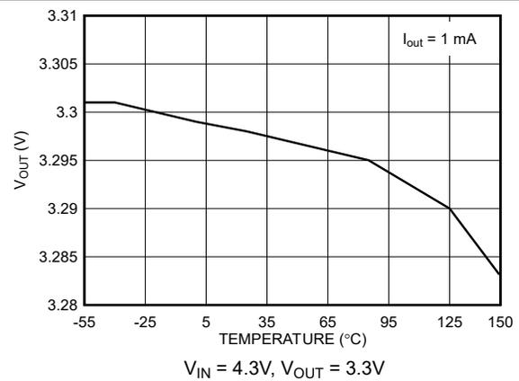
图 5-4. Output Voltage vs Temperature (New Chip)
