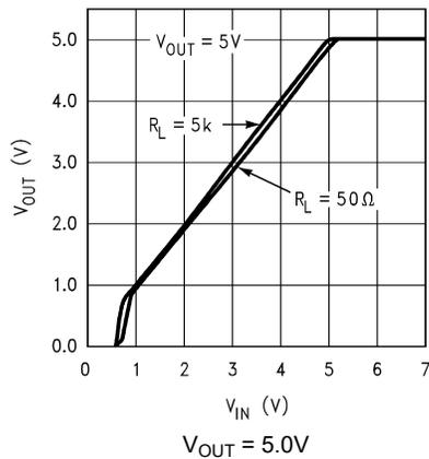
图 5-5. Output Voltage vs  $V_{IN}$  (Legacy Chip)
