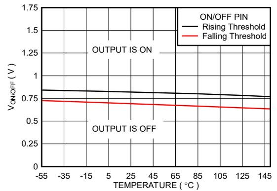
5-58.  $\overline{\text{ON/OFF}}$  Threshold vs Temperature (New Chip)
