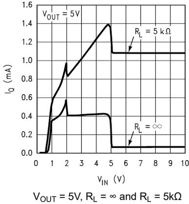
图 5-19. Input Current vs Input Voltage ( $V_{IN}$ ) (Legacy Chip)
