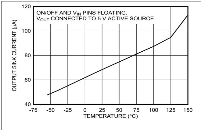
图 5-49. Output Reverse Leakage vs Temperature (New Chip)
