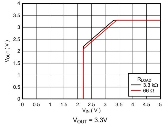
Figure 5-8. Output Voltage vs  $V_{IN}$  (New Chip)
