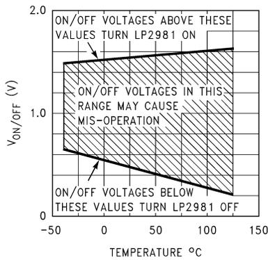
5-57.  $\overline{\text{ON/OFF}}$  Threshold vs Temperature (Legacy Chip)
