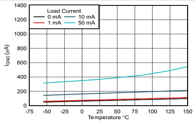
5-16. Ground Pin Current ( $I_{GND}$ ) vs Temperature (New Chip)
