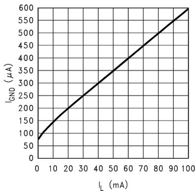
5-17. Ground Pin Current ( $I_{GND}$ ) vs Load Current (Legacy Chip)
