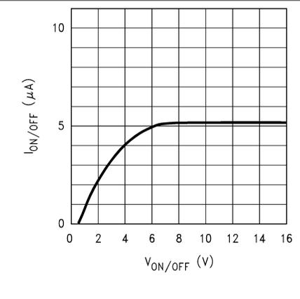
图 5-54.  $\overline{\text{ON/OFF}}$  Pin Current vs  $V_{\text{ON/OFF}}$  (Legacy Chip)
