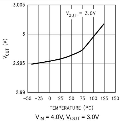
图 5-3. Output Voltage vs Temperature (Legacy Chip)
