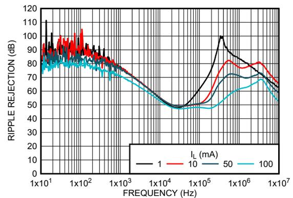
5-42. Ripple Rejection vs Load Current ( $I_L$ ) and Frequency (New Chip)
