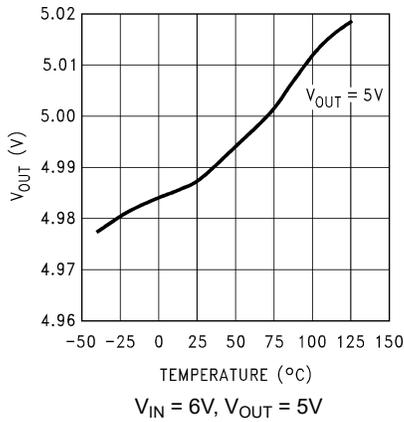
图 5-1. Output Voltage vs Temperature (Legacy Chip)
