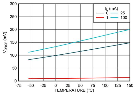
Figure 5-12. Dropout Voltage ( $V_{DO}$ ) vs Temperature (New Chip)
