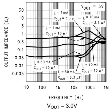
5-40. Output Impedance vs Frequency (Legacy Chip)
