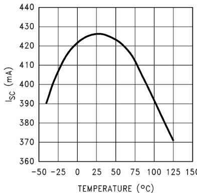
5-35. Instantaneous Short-Circuit Current vs Temperature (Legacy Chip)
