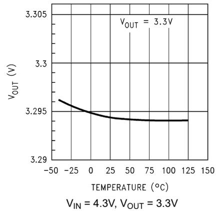
图 5-2. Output Voltage vs Temperature (Legacy Chip)
