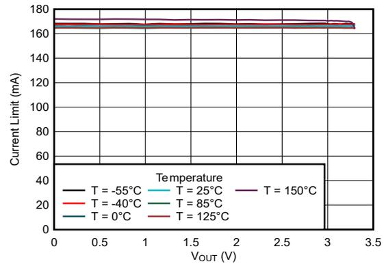
5-38. Short-Circuit Current vs Output Voltage ( $V_{OUT}$ ) (New Chip)
