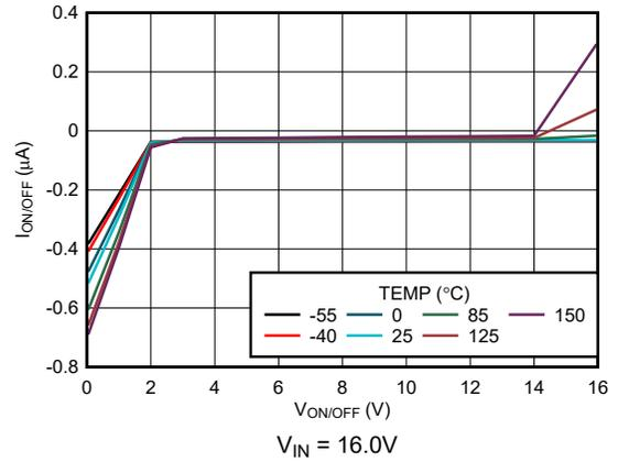
5-56.  $\overline{\text{ON/OFF}}$  Pin Current vs  $V_{\overline{\text{ON/OFF}}}$  (New Chip)
