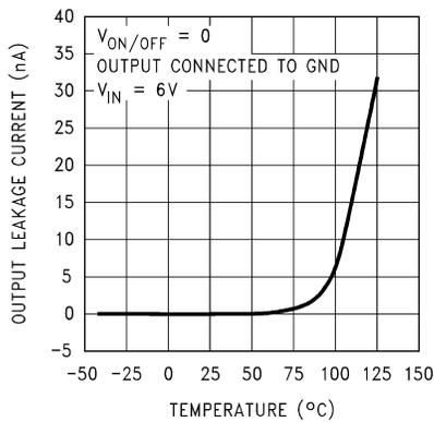
5-47. Input-to-Output Leakage vs Temperature (Legacy Chip)
