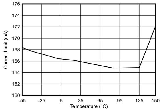
5-36. Instantaneous Short-Circuit Current vs Temperature (New Chip)
