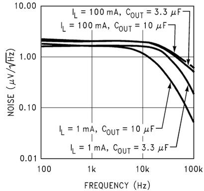
5-44. Output Noise Density vs Frequency (Legacy Chip)
