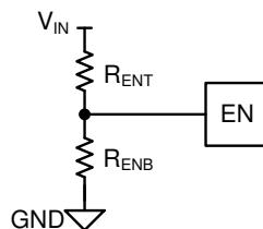
**图 8-5. Enable Divider to Set External UVLO Threshold**
