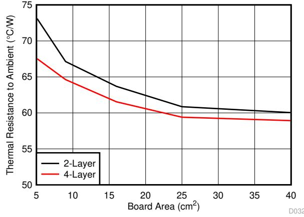
**図 8-48. Package Thermal Resistance vs Board Copper Area**
