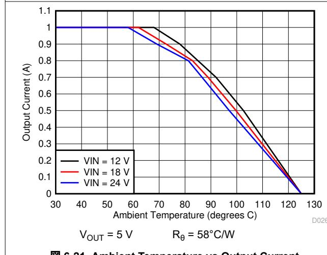
图 6-21. Ambient Temperature vs Output Current
