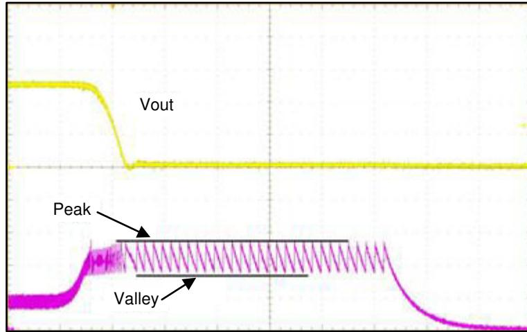
**图 7-1. Current Limit Operation During Output Short Circuit**
