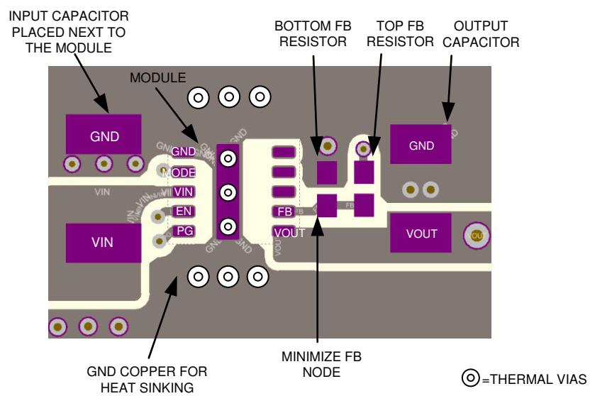
**图 8-50. Layout Example With Adjustable Output Version**
