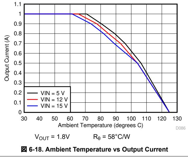
图 6-18. Ambient Temperature vs Output Current
