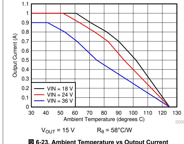
图 6-23. Ambient Temperature vs Output Current
