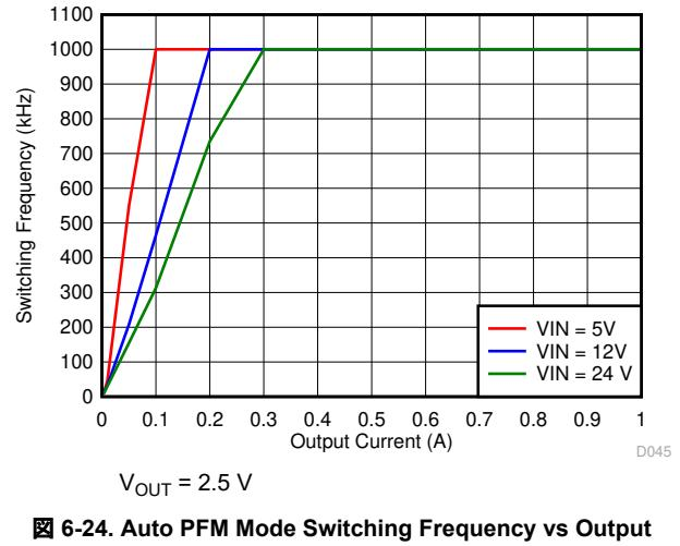
图 6-24. Auto PFM Mode Switching Frequency vs Output Current
