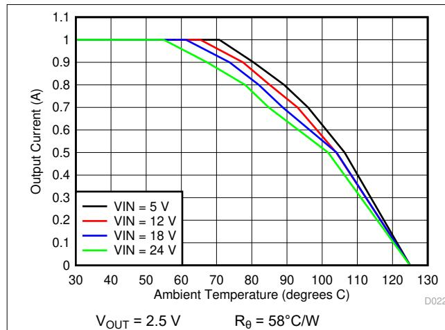
图 6-19. Ambient Temperature vs Output Current
