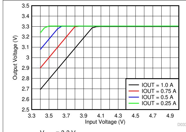
$V_{OUT} = 3.3\text{ V}$
