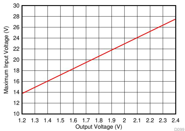
**图 8-3. Maximum Input Voltage for  $V_{OUT} < 2.5$  V**
