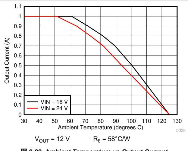
图 6-22. Ambient Temperature vs Output Current
