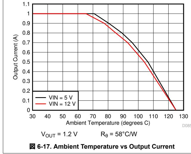
图 6-17. Ambient Temperature vs Output Current
