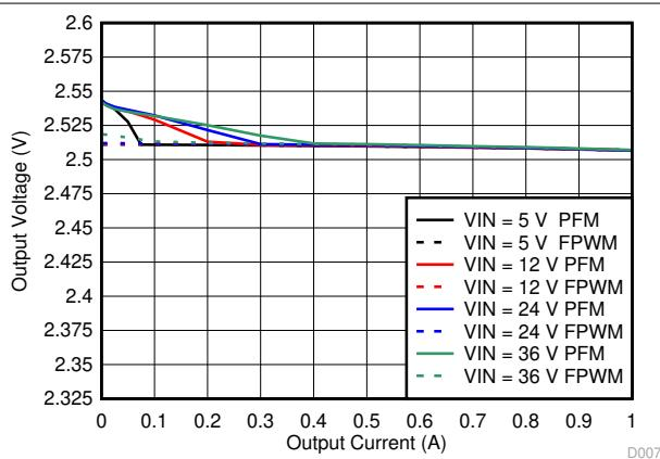
**図 8-34. Line and Load Regulation**
