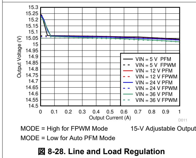
图 8-28. Line and Load Regulation
