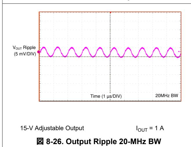
图 8-26. Output Ripple 20-MHz BW
