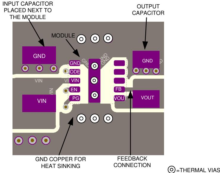
**図 8-49. Layout Example With Fixed Output Version**
