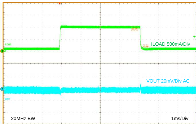
Figure 60. Load Transient V_{OUT} = 3.3\text{ V}
