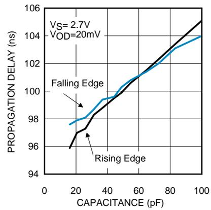
Figure 10. Propagation Delay vs. Capacitive Load
