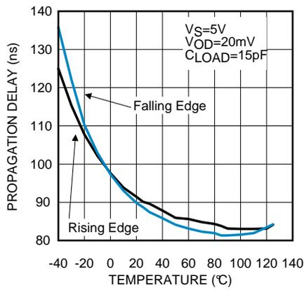
Figure 9. Propagation Delay vs. Temperature
