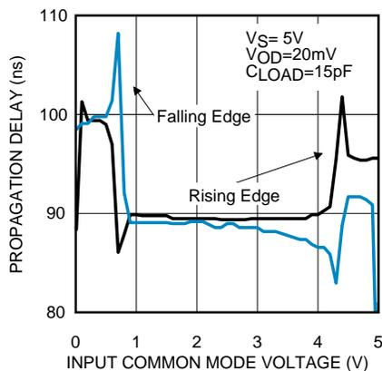
Figure 15. Propagation Delay vs. Common-Mode Voltage
