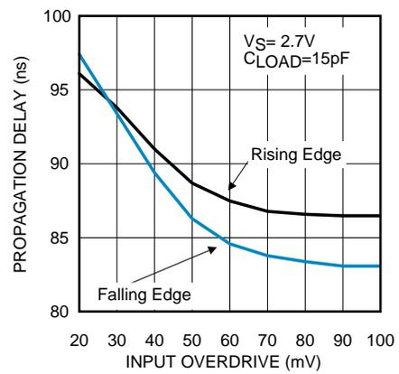
Figure 12. Propagation Delay vs. Input Overdrive
