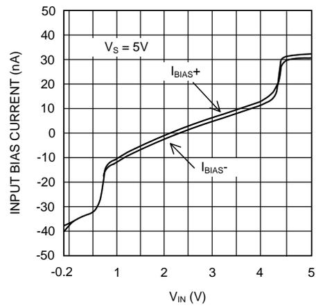
Figure 6. Input Bias Current vs. Input Voltage
