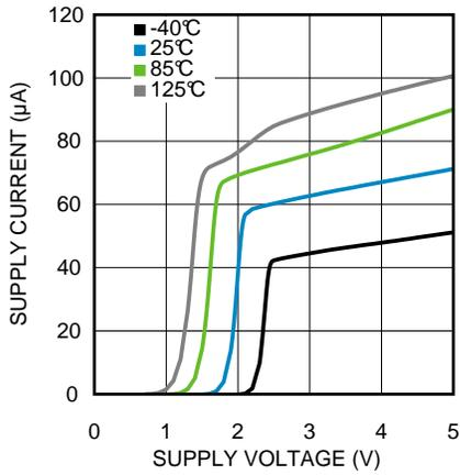
Figure 1. Supply Current vs. Supply Voltage
