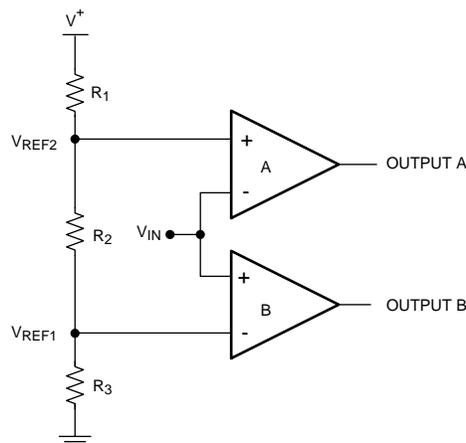
Figure 29. Window Detector
