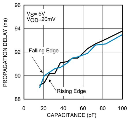
Figure 11. Propagation Delay vs. Capacitive Load
