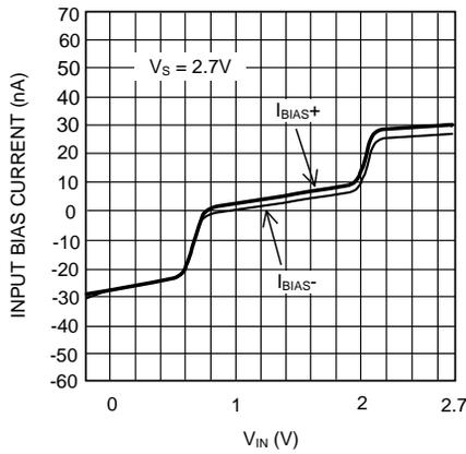
Figure 7. Input Bias Current vs. Input Voltage
