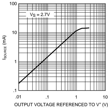
Figure 3. Sourcing Current vs. Output Voltage
